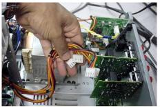
All four connectors from P6810, P6812, P6008A and P6008B are disconnected to give ease of movement for the power amplifier module.
