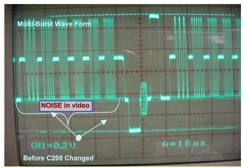
In HT-R500 a change in C205 from its current value 100uf16V capacitor to 1000/6.3V will help eliminate the ringing and jitter in video waveform.
