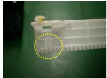
Align the long tooth on the rack (see left) with the half tooth on the gear (see right)
