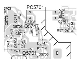
Step 2: Replace the chip resistor, R5729 with discrete part (ERDS2TJ562T) by back-solder. Connect the discrete resistor from pin 1 of PC5701 to ground by wire (REU35R055CC). Apply bond after the back-solder of the part.
