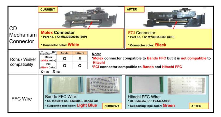
Caution: If the old 30P Connector (K1MN30B00046) is used in the product and the replacement of 30P FFC is required, please use the 30P FFC kit and replace the 30P FFC and 30P Connector at the same time.
