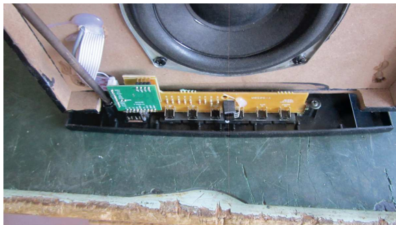
1. Disassemble the screws on control board.
