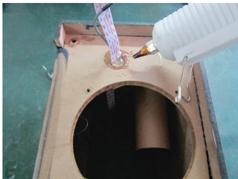
3. Assemble the cables in subwoofer.
