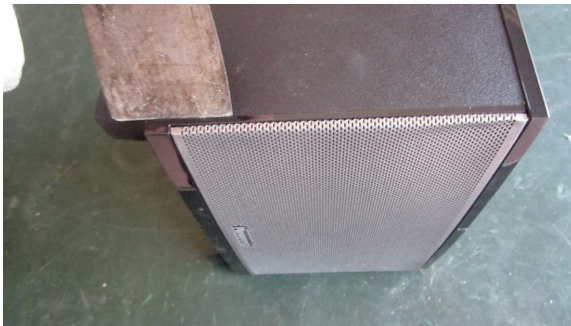
1. Disassemble the front metal cover with the tool as shown.
