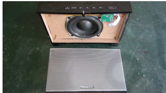
2. After metal cover being disassembled.
