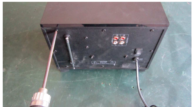
2. Disassemble the screws on back panel.
