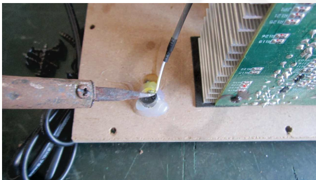
5. Disassemble the antenna with the soldering tool as shown.
