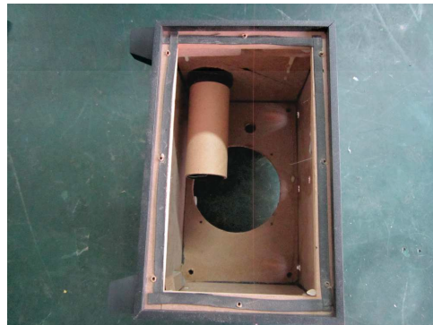
2. Assemble the EVA pad on subwoofer wooden box.
