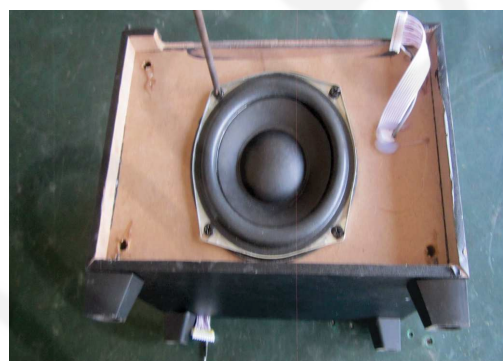
4. Assemble the screws of speakers.
