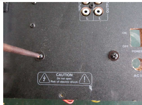
6. Assemble the screws of transformer.
