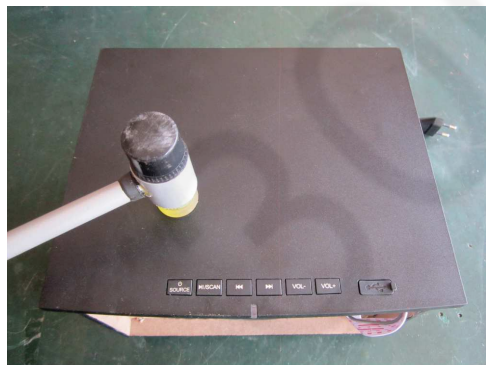
12. Assemble the top plastic panel.
