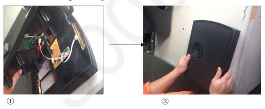
Step1: Insert the cable into the connector, then close the top panel and middle frame
