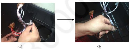
Step 7: As above picture ①-② shown, Insert the 7pin cable to control board PCBA, 8Pin cable to Input-Output PCBA
