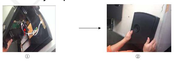
Step1: Insert the cable to the connector, then close the top panel and middle frame
