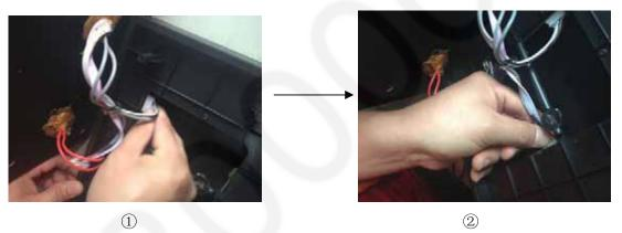
Step 8: As above picture ①-② shown, Insert the 7pin cable to control board PCBA, 8Pin cable to Input-Output PCBA
