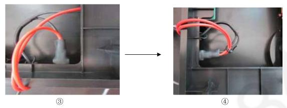
Step 7: As above picture ①-④ shown, Twist the main cord of woofer middle frame and transformer primary fuses of wooden box together, take a cable connector to link them together. Then thread the transformer primary fuses which with terminal end through into the heat-shrinkable tubing, and insert it on power switch. Use a Heat Gun to heat the heat-shrinkable tube to make it wrap the power switch tightly
