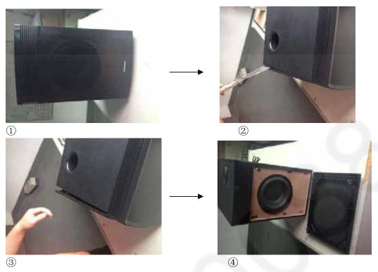
Step 1: Insert the knife into the grooves of front panel assembly. Push the steel rule forward and backward as shown above from  $\bigcirc$ - $\bigcirc$
