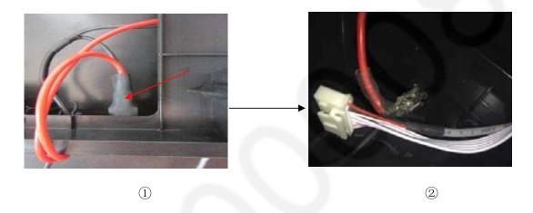
Step 3: Use a scissor to cut the heat-shrinkable tube, Press the key by using a tool with a sharp point as above arrow shown, then pull out the red cable.
