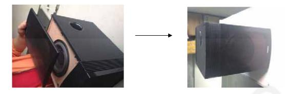
Step 10: As shown in the picture, Install metal grill to wooden box.
