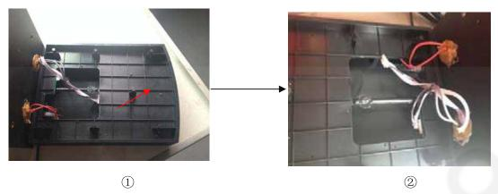
Step 2: Detach the 8 pin and 7pin cable away from middle frame as above arrow shown from 1- 2.
