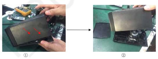
Step 2: As shown in above picture ①, One hand grab the back panel of satellite unit, then another hand grab the middle frame outward force to detach the middle frame and back panel. Then the satellite top panel will come off automatically as shown in picture ②.
