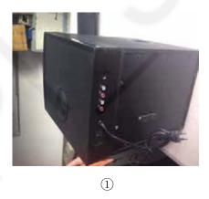
Step 9: As shown in the picture, Cover the top panel on wooden box, then use rubber hammer to install it well.
