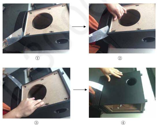
Step 1: Upset the speaker unit as shown above, Insert the knife into the grooves of middle frame assembly. One hand press the speaker box, the other hand push the steel rule forward and backward as shown above from ①-④
