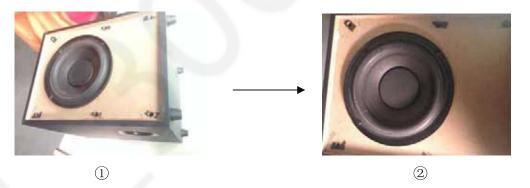
Step 4: Put the speaker on wooden box, then use 4 screws to fix the speaker.
