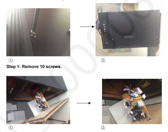
Step 2: take out the back panel from wooden box , then detach 4 cable line away from PCB  $\,$
