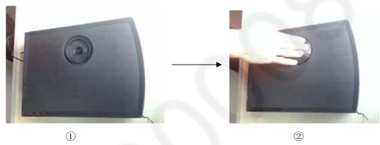
Step 3: Install the knob on Top panel.
