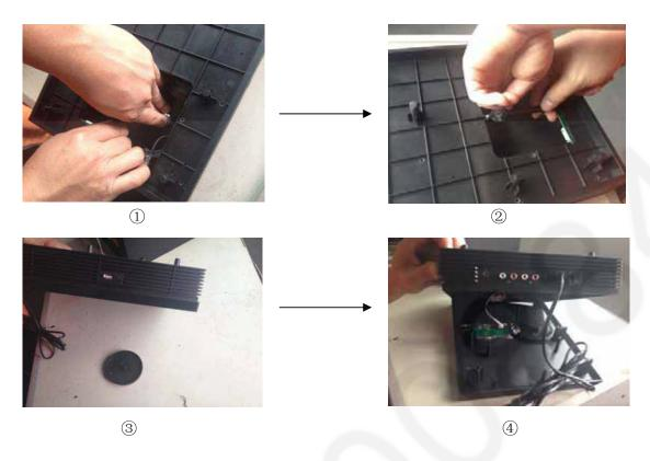
Step 5: One hand press and hold the bottom of frame, then another hand, grab the connecting rod outward force to detach the middle frame and top panel. Then the volume knob will come off from top panel automatically.
