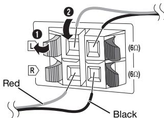
**Be careful not to cross (short-circuit) or reverse the polarity of the speaker wires as doing so may damage the speakers.**
