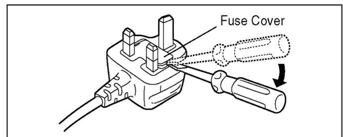
2. Replace the Fuse and attach the Fuse cover.
