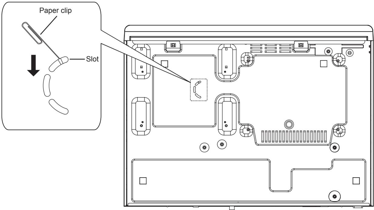
4. Put the unit upward, and pull out the tray.
