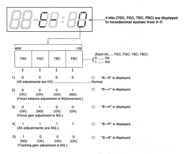
Note: If any other disc than the test disc (SZZP1054C) is used, an "E-8" may be displayed.
