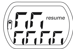
test pattern 2 (alternate segments activated)
