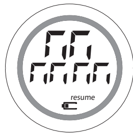
test pattern 2 (alternate segments activated)
