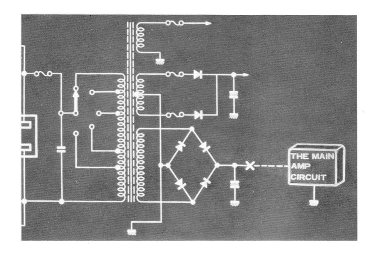
REPLACE THE BLOWN FUSE AND APPLY POWER TO THE UNIT.
