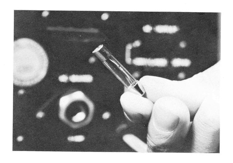
6. IN CASE THE FUSE BLOWS, HOW THE FUSE BLOWS WILL ALSO TELL US THE NATURE OF THE PROBLEM.
