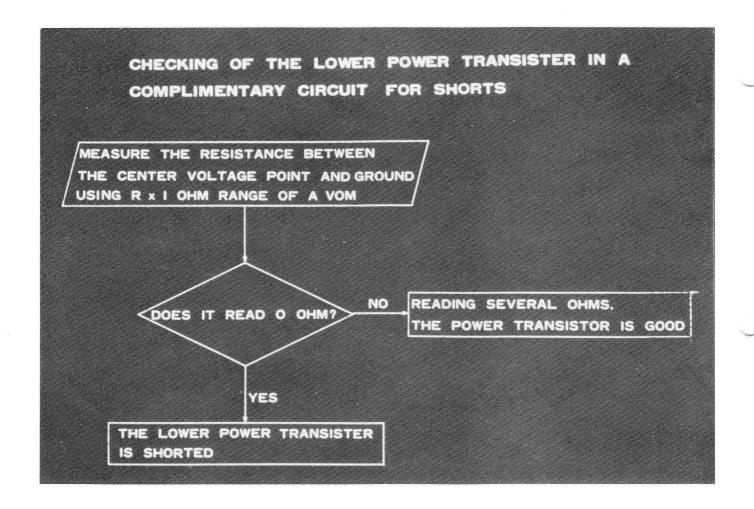
CHECKING THE LOWER POWER TRANSISTOR IN A COMPLIMENTARY
