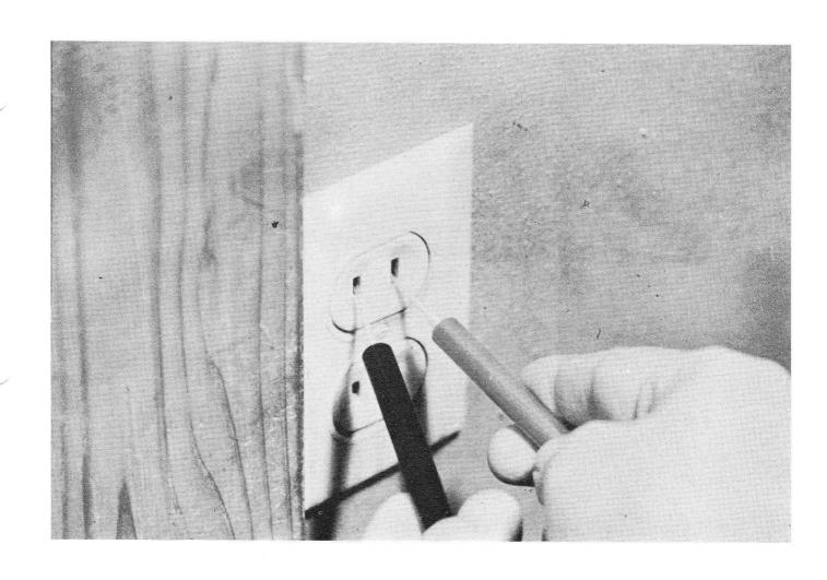
13. MEASURE THE LINE VOLTAGE TO SEE IF YOU ARE GETTING AC VOLTAGE OUT OF THE CORD. USE A VTVM ON 250V SCALE.
