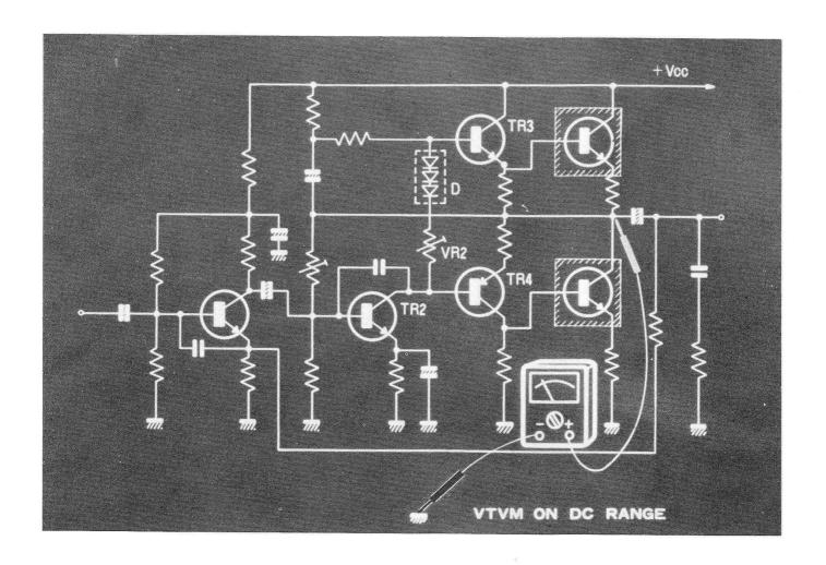
46. A VOLTAGE READING LOWER THAN ½ VCC INDICATES A FAILURE OF TR-2 OR TR-4.
