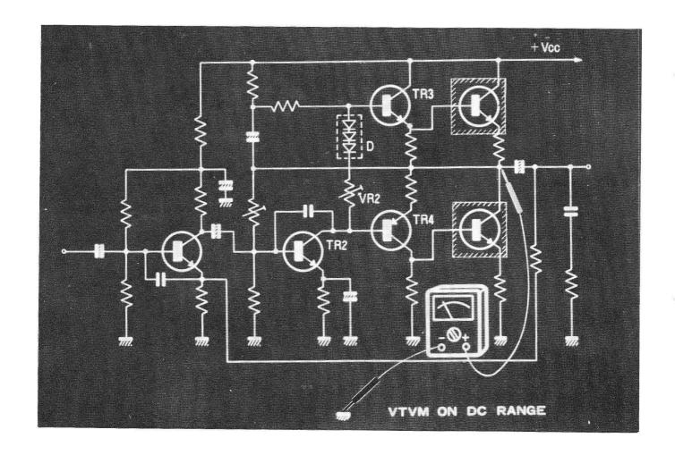
IF YOU DO HEAR BUZZING, THEN EXCESSIVE CURRENT MUST BE FLOWING THROUGH THE DRIVER STAGE.
