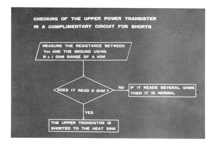
32. CHECKING THE UPPER POWER TRANSISTOR IN A COMPLIMENTARY CIRCUIT.
