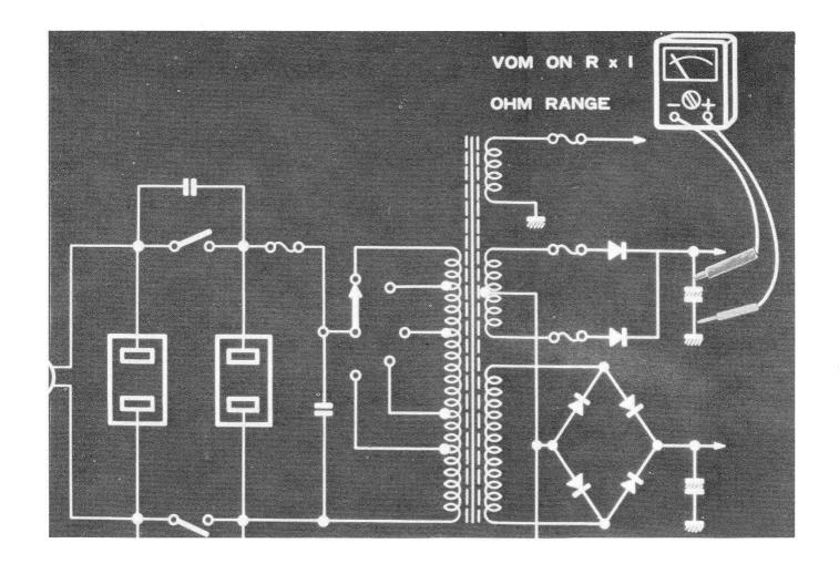
IF THEY CHECK OK, THEN TEST THE FILTER CAPACITORS BY PLACING YOUR VOM ON THE Rx1 OHM RANGE, AND PLACE THE TEST LEADS ACROSS THE CAPACITOR. IF THE CAPACITOR IS GOOD, YOUR METER WILL SWING FROM INFINITY TO ZERO AND SLOWLY RETURNS TO INFINITY AGAIN. IF THE CAPACITOR IS SHORTED, IT WILL READ CONSTANT ZERO OR VERY SMALL RESISTANCE.
