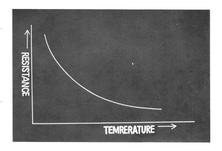
A GOOD TEMPERATURE COMPENSATING DIODE DECREASES RESIST-ANCE WITH INCREASING TEMPERATURE AND THEREFORE COM-PENSATE THE BIAS OF THE TRANSISTORS IT IS CONNECTED TO.
