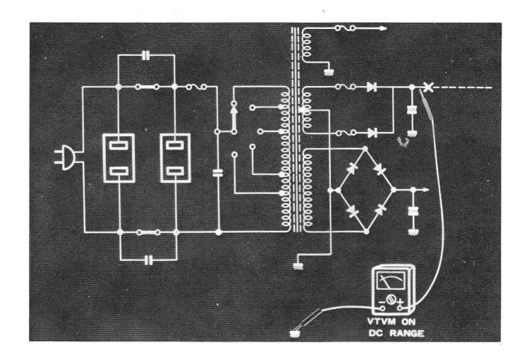
TO DETERMINE IF THE PROBLEM IS IN THE RECTIFIER SIDE OR THE LOAD SIDE OF THE POWER SUPPLY, REMOVE THE B(+) LINE WHICH IS CONNECTING THE LOAD TO THE POWER SUPPLY.
