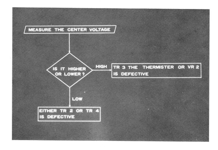
47. MEASURE THE CENTER VOLTAGE. IS IT HIGHER OR LOWER THAN ½ VCC? IF IT IS HIGHER THEN TR-3, THE THERMISTER OR VR2 IS DEFECTIVE. IF IT IS LOWER, THEN TR2 OR TR4 IS DEFECTIVE.
