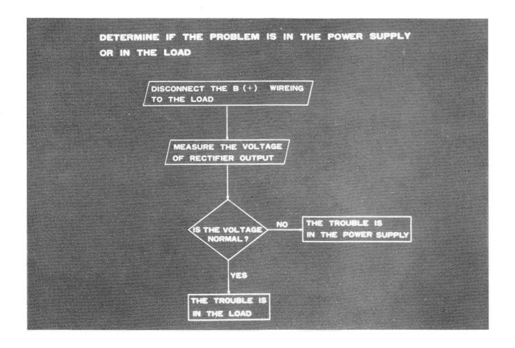
DETERMINE IF THE PROBLEM IS IN THE POWER SUPPLY OR IN THE LOAD.
