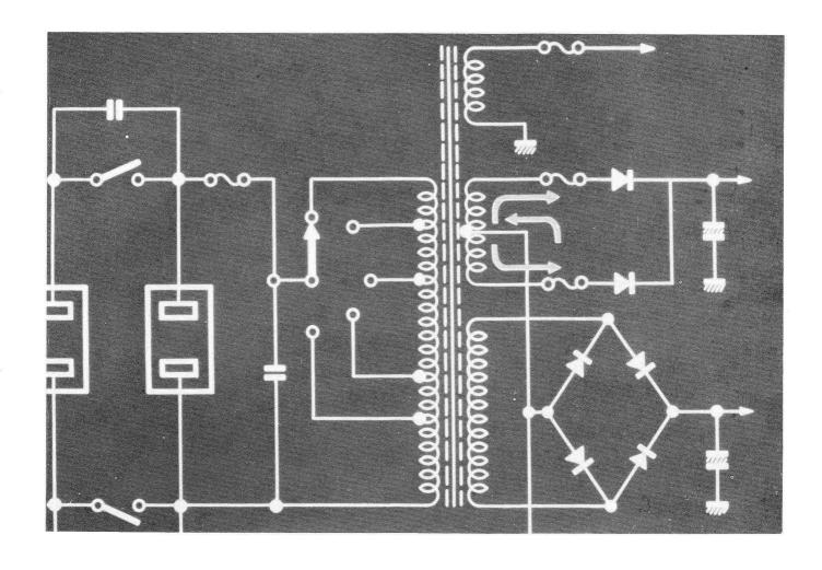
49. HERE AGAIN THE PROBLEM MAY BE IN THE POWER SUPPLY. THE SECONDARY SIDE OF THE POWER TRANSFORMER MAY BE OVER-LOADED.
