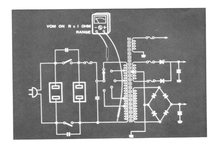
TO CHECK THE PRIMARY WINDING, UNPLUG THE MAIN POWER FROM THE WALL, THEN MEASURE THE CONTINUITY ACROSS THE PRIMARY WINDING-USING A VOM ON Rx1 OHM RANGE. WHENEVER YOU CHECK THE CONTINUITIES, PLEASE BE SURE TO UNPLUG THE AC CORD FROM THE WALL. YOU SHOULD GET A READING OF APPROXIMATELY 30-300 OHMS. IF THE READING IS INFINITY THEN THE PRIMARY WINDING IS OPEN.
