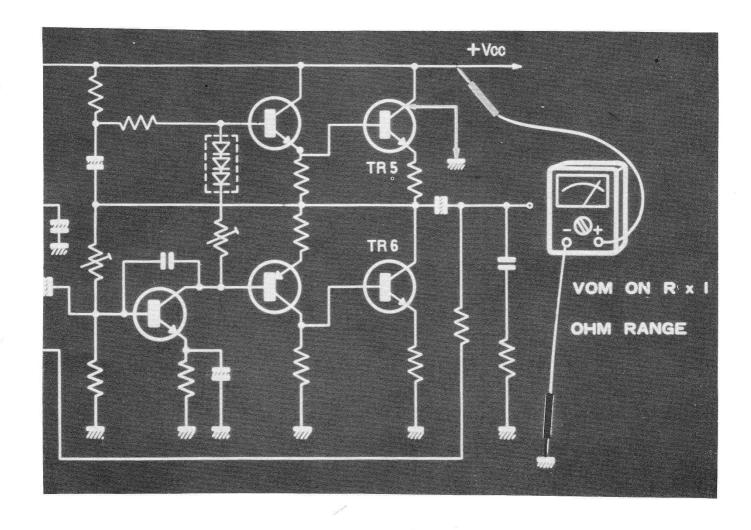
TO LOCATE THE PROBLEM, MEASURE THE RESISTANCE FROM VCC TO GROUND. YOUR VOM SHOULD BE SET ON Rx1 OHM RANGE. ZERO RESISTANCE INDICATES A SHORT TO THE HEAT SINK OF TR5. IN THIS MEASUREMENT, THE POWER SUPPLY CIRCUIT SHOULD BE DISCONNECTED WITH THE MAIN AMP CIRCUIT.
