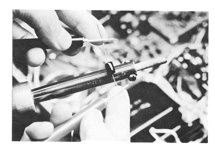
TO CHECK THESE DIODES JUST USE YOUR VOM ON THE Rx1 OHM RANGE. CHECK THE RESISTANCE IN A FORWARD BIAS DIRECTION WHILE YOU HEAT THE DIODE WITH YOUR FINGER OR SOLDERING IRON. IF THE RESISTANCE DECREASES AS THE TEMPERATURE RISES THEN THE DIODE IS GOOD. IF THE RESISTANCE DOES NOT CHANGE, IT IS DEFECTIVE.
