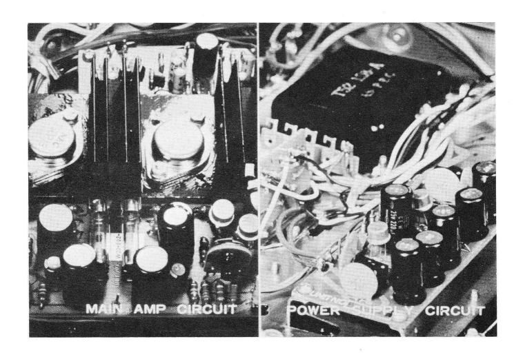
WHEN THE FUSE DOES NOT BLOW, THE TROUBLE IS IN THE POWER SUPPLY CIRCUIT IN MOST CASES. HOWEVER, WHEN THE FUSE BLOWS THEN THE GENERAL CASE OF THE TROUBLE WILL BE IN EITHER THE POWER SUPPLY OR THE MAIN AMP CIRCUIT.
