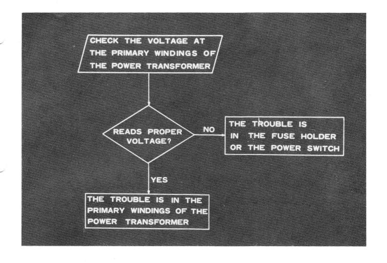
17. CHECK THE VOLTAGE AT THE PRIMARY WINDING OF THE TRANS-FORMER. IF IT READS THE PROPER VOLTAGE THEN THE PRIMARY WINDING IS DEFECTIVE. IF IT DOES NOT READ PROPERLY THEN THE FUSE HOLDER OR THE POWER SWITCH IS DEFECTIVE.
