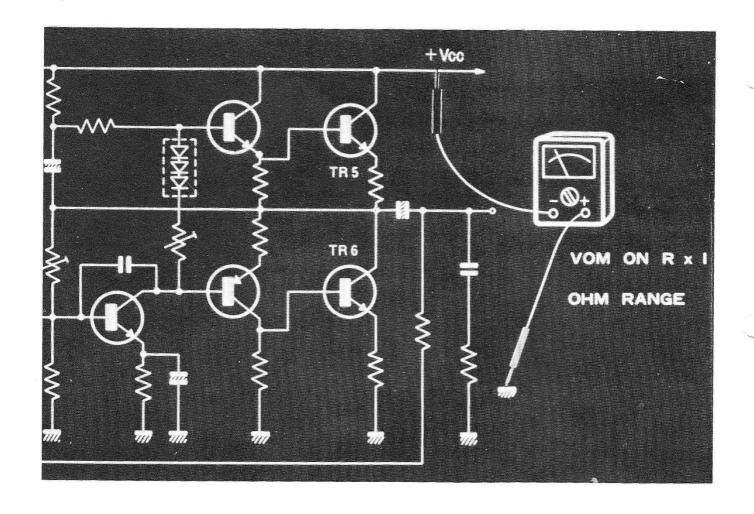
NOW REVERSE THE POLARITY OF THE TEST LEADS AND TAKE ANOTHER READING. IF THIS READING IS EQUAL TO THE SUM OF BOTH EMITTER RESISTORS THEN BOTH TRANSISTORS ARE SHORTED.
