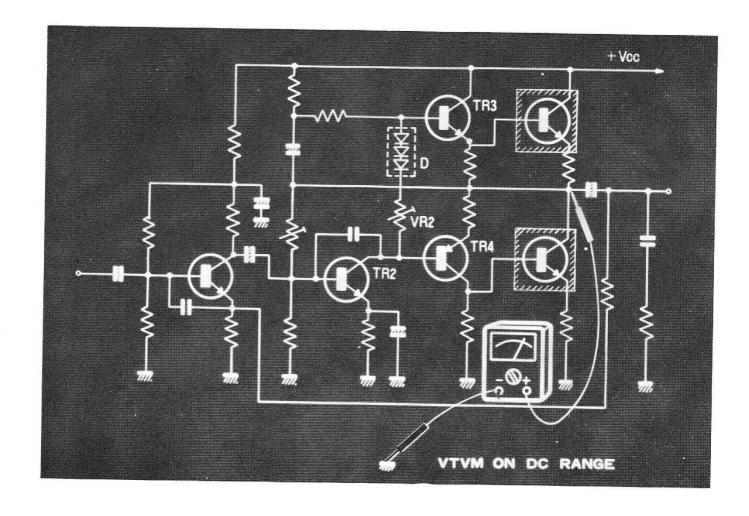
45. IF THE VOLTAGE READING IS HIGHER THAN ½ VCC, THEN TR-3 IS DEFECTIVE, OR THE TEMPERATURE COMPENSATING ELEMENT OR VR2 IS OPEN.
