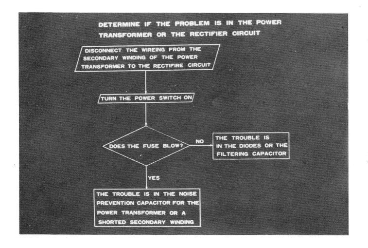
DETERMINE IF THE PROBLEM IS IN THE POWER TRANSFORMER OR THE RECTIFIER CIRCUIT. DISCONNECT THE WIRING FROM THE SECONDARY WINDING OF THE POWER TRANSFORMER TO THE RECTIFIER CIRCUIT. TURN THE POWER SWITCH ON, DOES THE FUSE BLOW? IF "YES", THE TROUBLE IS IN THE NOISE PREVENTION CAPACITOR FOR THE POWER TRANSFORMER OR A SHORTED SECONDARY WINDING. IF "NO," THE TROUBLE IS IN THE DIODES OR THE FILTER CAPACITOR.
