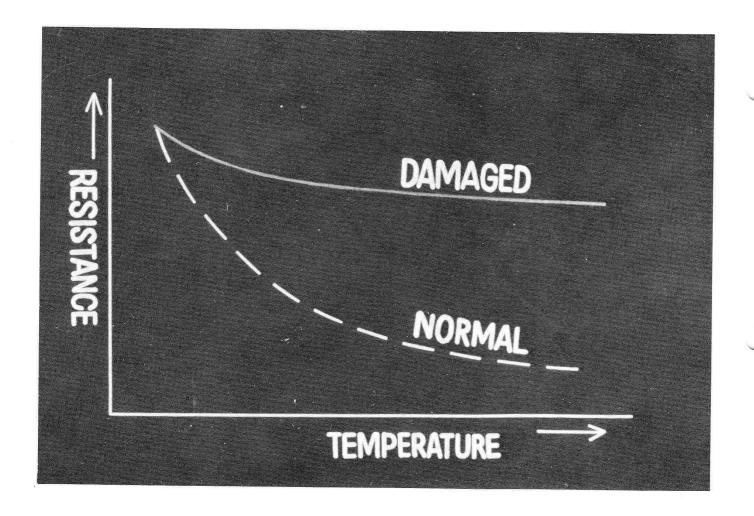
IF A DIODE IS DAMAGED, ITS RESISTANCE VALUE WILL NOT CHANGE
