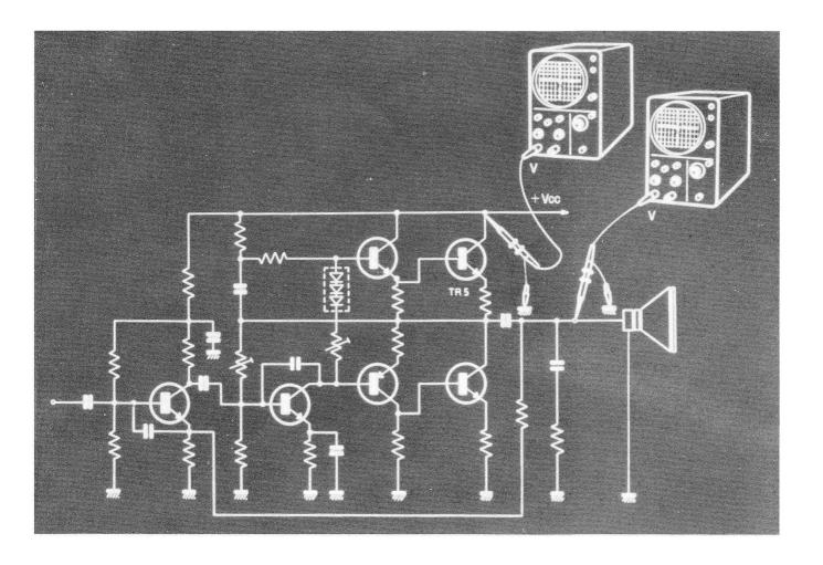
WHEN YOU HEAR BUZZING OF THIS NATURE, IT IS A GOOD INDICA-TION THAT THE UPPER TRANSISTOR TR5 IS SHORTED. THIS CAN BE VERIFIED WITH AN OSCILLOSCOPE.
