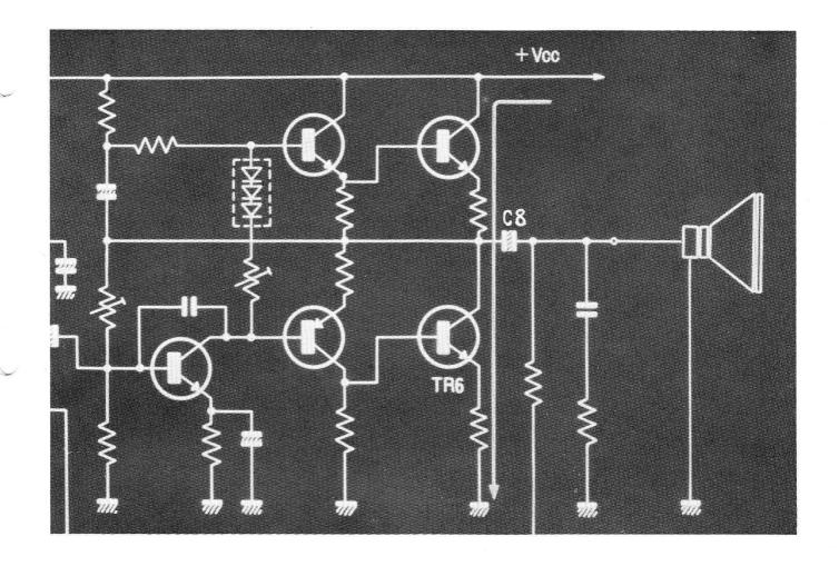
41. THIS IS BECAUSE INSTEAD OF THE RIPPLE COMPONENT GOING THROUGH C-8 AND THE SPEAKER, IT GOES RIGHT THROUGH TR-6 AND R-15 TO GROUND.
