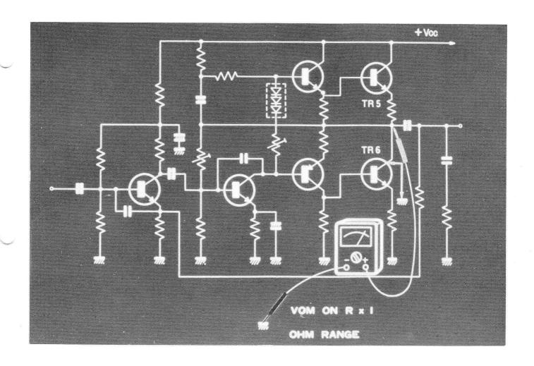
TO CHECK THE LOWER POWER TRANSISTOR, MEASURE THE RESIST-ANCE BETWEEN THE CENTER AND GROUND WITH A VOM SET ON THE Rx1 OHM RANGE. A ZERO READING INDICATES A SHORTED LOWER TRANSISTOR.
