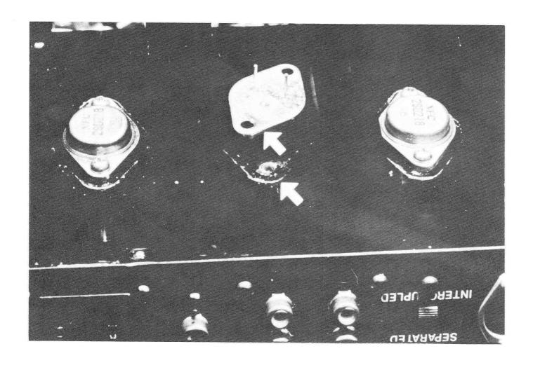
AS AN EXAMPLE WE WILL LOOK AT THE SYMPTOMS OF A SHORT CIRCUIT BETWEEN THE COLLECTOR OF A POWER TRANSISTOR AND THE HEAT SINK ITS MOUNTED UPON.
