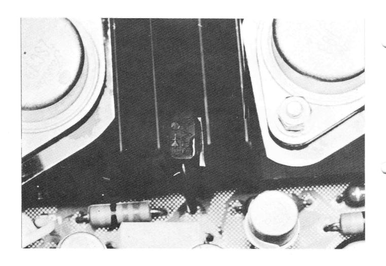
HERE YOU WILL SUSPECT THE TEMPERATURE COMPENSATING DIODES ARE DEFECTIVE. THEY SHOULD CHANGE VALUE ACCORDING TO THE TEMPERATURE BUT DEFECTIVE ONES WILL NOT.
