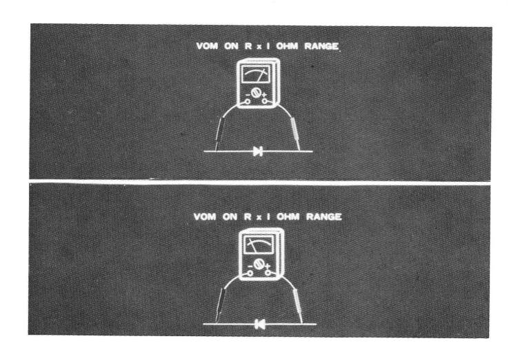
TO CHECK DIODES, SET THE VOM ON Rx1 OHM RANGE AND PLACE
