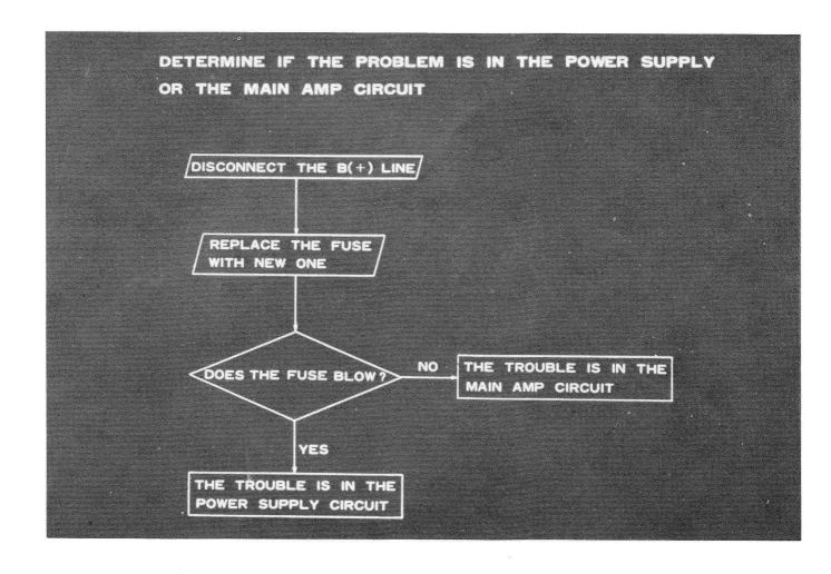
DETERMINE IF THE PROBLEM IS IN THE POWER SUPPLY OR THE MAIN AMP CIRCUIT. DISCONNECT THE B(+) LINE, REPLACE THE BLOWN FUSE. DOES THE FUSE BLOW AGAIN? IF "YES", THE PROBLEM IS IN THE POWER SUPPLY. IF "NO", THE PROBLEM IS IN THE MAIN AMP CIRCUIT.
