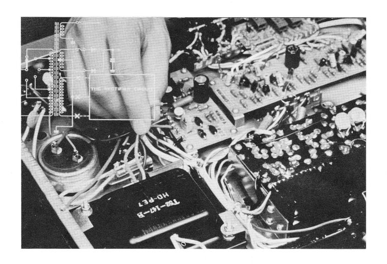
TO CHECK THE POWER SUPPLY CIRCUIT, DISCONNECT THE RECTI-FIER CIRCUIT FROM THE SECONDARY WINDING OF THE TRANS-FORMER. TURN ON THE UNIT WITH A GOOD FUSE INSTALLED. IF THE FUSE BLOWS THE FAILURE IS IN THE TRANSFORMER OR THE NOISE PREVENTION CAPACITOR.
