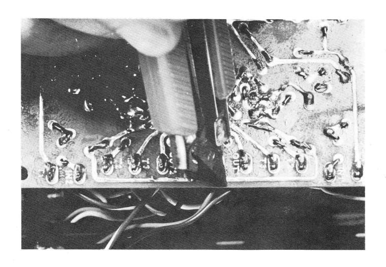
WHEN YOU CHECK UNITS THIS WAY, IT CAN BE VERY HELPFUL TO LOCATE THE PROBLEM FROM THE NEIBORHOOD OF THE RECTIFIER CIRCUIT THEN ON TO THE LOAD.
