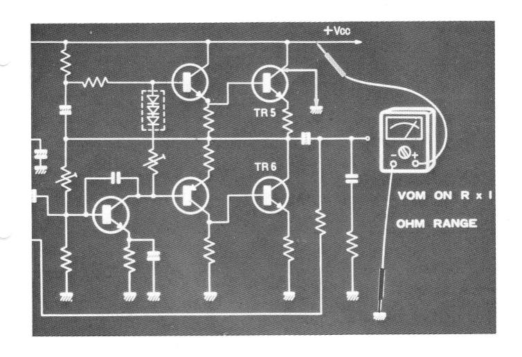
NOW WE WILL CONSIDER A CASE WHERE A SHORT OCCURS BETWEEN THE COLLECTOR AND EMITTER IN BOTH TRANSISTORS AT THE SAME TIME. USE YOUR VOM SET ON Rx1 OHM RANGE AND TAKE A READING.
