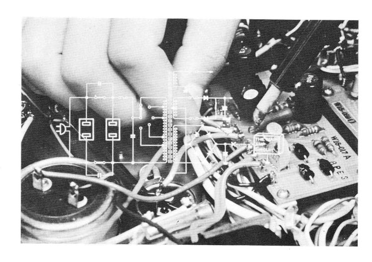
21. TO DETERMINE IF THE PROBLEM IS IN THE POWER SUPPLY OR THE MAIN AMP CIRCUIT, DISCONNECT THE B(+) LINE TO THE MAIN AMP.
