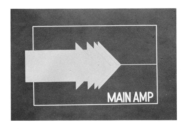
29. IF THE PREVIOUS TEST HAVE NOT LOCATED THE PROBLEM THEN THE FAULT IS PROBABLY IN THE MAIN AMP CIRCUIT DUE TO EXCESSIVE CURRENT FLOWING INTO THE MAIN AMP.
