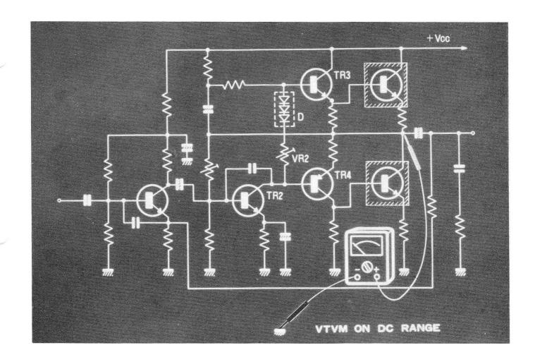
43. IF YOU DO NOT HEAR BUZZING THEN MEASURE THE CENTER VOLTAGE. IF IT READS EXACTLY ½ OF VCC THEN THE CIRCUIT IS WORKING NORMAL. YOU CAN SUSPECT THAT EITHER ONE OF THE POWER TRANSISTORS YOU JUST REMOVED IS DEFECTIVE.
