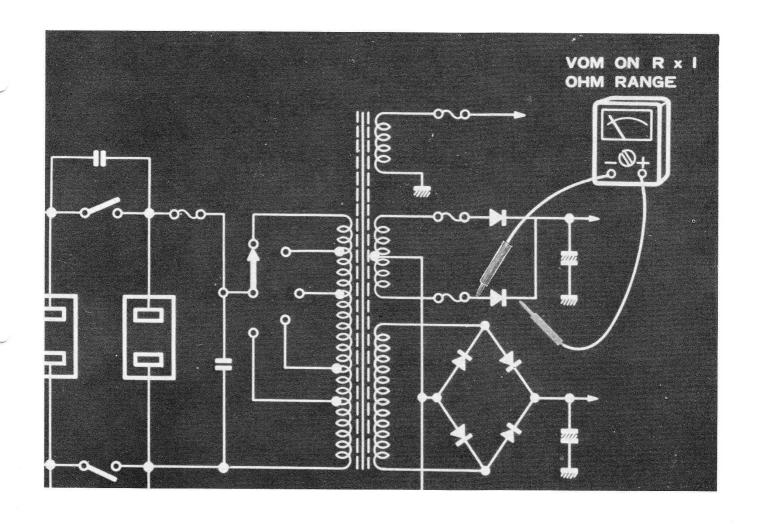
55. IF THE FAILURE IS IN THE POWER SUPPLY, THEN INSURE THAT THE POWER IS OFF AND CHECK THE DIODES FOR SHORTS.
