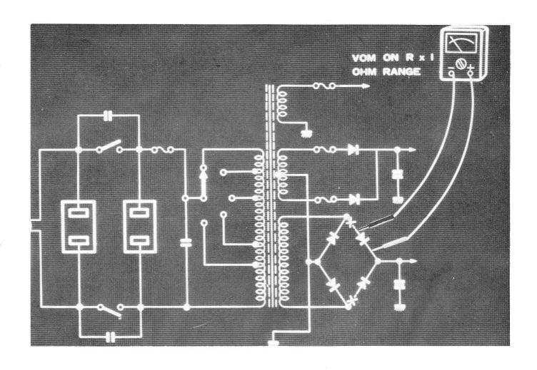
25. IF THE FUSE DID NOT BLOW IN THE PREVIOUS CHECK, THEN YOUR NEXT STEP IS TO CHECK THE DIODES IN THE RECTIFIER CIRCUIT FOR SHORTS.
