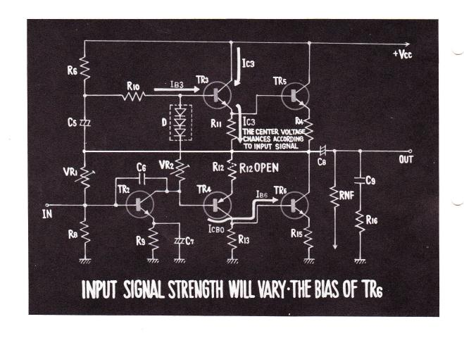
THIS  $I_{CEBO}$  OF TRANSISTOR 4 CHANGES DEPENDING UPON THE INPUT SIGNAL. ACCORDINGLY, THE BIAS VOLTAGE OF TRANSISTOR 6 ALSO CHANGES, THE CENTER VOLTAGE VARYING FROM HIGH TO NEAR 1/2  $V_{CC}$  IN ACCORDANCE WITH THE INPUT SIGNAL STRENGTH.
