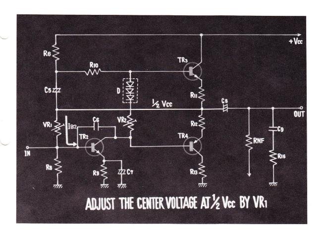
THUS, THE CENTER VOLTAGE CHANGES AS YOU CHANGE THE BIAS OF TRANSISTOR 2. SO THAT IF THE CENTER VOLTAGE IS SET AT  $1/2~V_{CC}$  BY ADJUSTING VR<sub>1</sub>, THEN THE CENTER VOLTAGE CAN ALWAYS BE MAINTAINED AT  $1/2~V_{CC}$  BY MEANS OF THE DC FEEDBACK.
