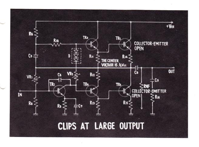
61. IN THIS CASE, NO ABNORMALITY OCCURS AT LEAST DC-WISE. THE CENTER VOLTAGE WILL BE KEPT AT A NORMAL VALUE OF 1/2  $V_{\text{CC}}$ . FROM THE VIEWPOINT OF AC, THERE IS NO PROBLEM WHEN THE OUTPUT IS VERY SMALL. HOWEVER, LARGE OUTPUT CANNOT BE PRODUCED, DUE TO CLIPPING.
