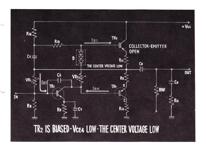
31. ACTUALLY, HOWEVER, VOLTAGE APPEARS AT THE CENTER POINT BY THE BASE CURRENT IN TRANSISTOR 3.
