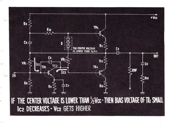
15. NOW, LET'S CONSIDER THE CASE WHERE THE CENTER VOLTAGE HAS DECREASED AND HAS BECOME LOWER THAN  $1/2\ V_{C\,C}$ . THE BIAS VOLTAGE FOR TRANSISTOR 2 BECOMES INSUFFICIENT, BECAUSE OF THE DIRECT-CURRENT FEEDBACK FROM THE CENTER POINT THROUGH VR<sub>1</sub> TO TRANSISTOR 2. THE COLLECTOR CURRENT, I<sub>C 2</sub>, DECREASES AND THE COLLECTOR VOLTAGE V<sub>C 2</sub> GETS HIGHER.
