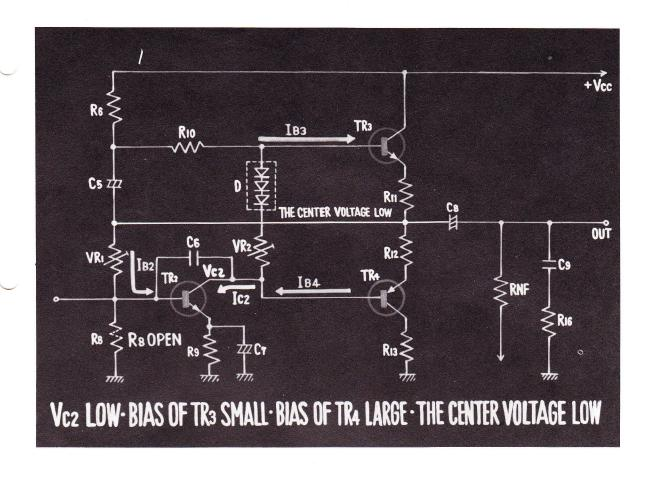
45. WHEN THE RESISTOR R<sub>8</sub> IS OPEN, THE BIAS VOLTAGE OF TRANSISTOR
