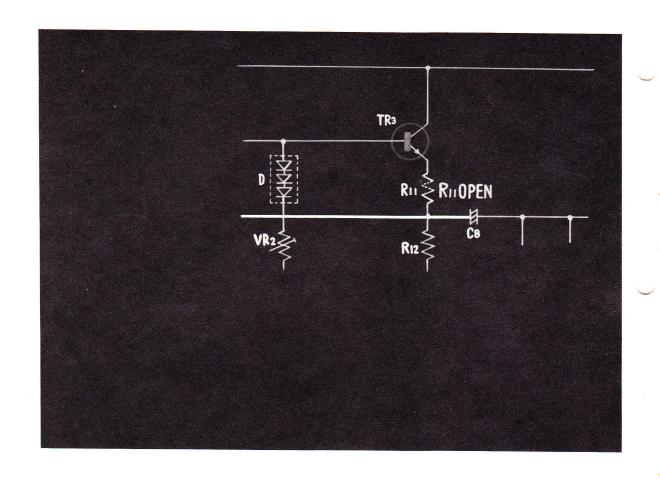
$^{50.}$  What about the case when the resistor  $\rm R_{1\,1}IS$  open?
