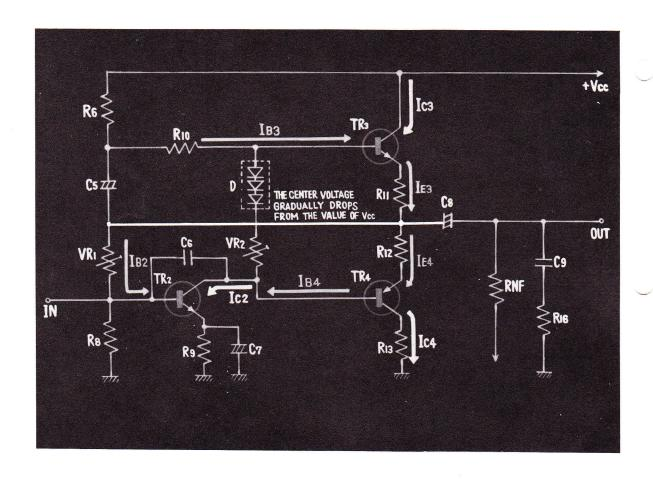
14. BUT AS TRANSISTOR 2 BEGINS TO FUNCTION, AND FURTHER, TRANSISTOR 4 FUNCTIONS, THE VOLTAGE OF THE CENTER POINT GRADUALLY DROPS FROM THE VALUE CLOSE TO  $V_{\text{CC}}$ .
