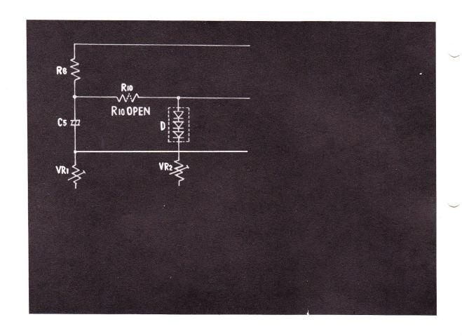
48. WHAT WILL HAPPEN WHEN THE LOAD RESISTOR  $R_{1\,0}$  OF TRANSISTOR 2 IS OPEN?
