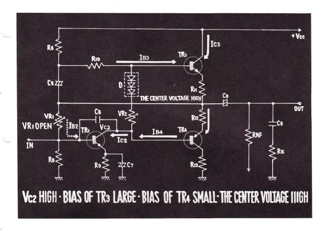
43. IF VR<sub>1</sub> IS OPEN, IT WILL NOT ALLOW TO GIVE BIAS VOLTAGE TO TRANSISTOR 2. THEREFORE, THE COLLECTOR CURRENT OF TRANSISTOR 2 DECREASES, CAUSING THE COLLECTOR VOLTAGE TO INCREASE.
