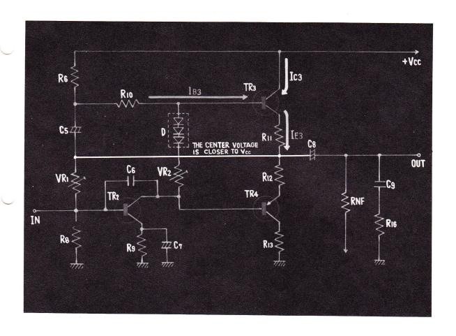
13. THE INSTANT  $V_{c\,c}$  IS APPLIED, THE VOLTAGE AT THE CENTER POINT BECOMES ALMOST AS HIGH AS  $V_{c\,c}$  ITSELF, BECAUSE A BIAS VOLTAGE IS GIVEN TO TRANSISTOR 3.
