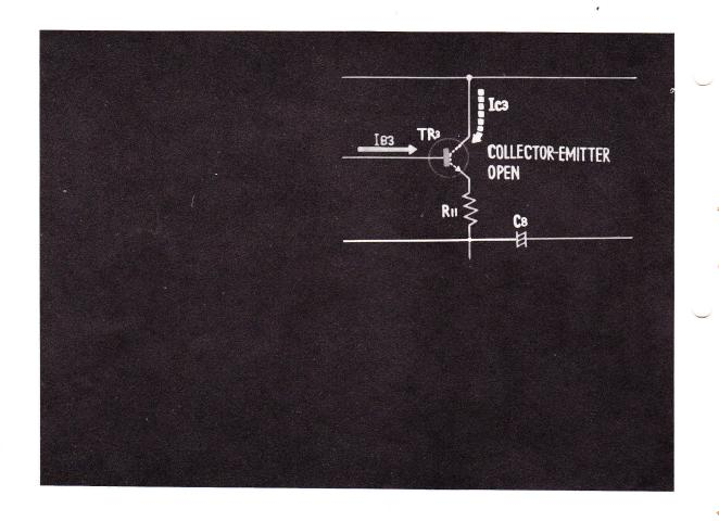
30. IT MAY SEEM THAT WHEN THE COLLECTOR AND THE EMITTER OF TRANSISTOR 3 IS OPEN, NO VOLTAGE WOULD APPEAR AT THE CENTER POINT, BECAUSE NO COLLECTOR CURRENT FLOWS TO TRANSISTOR 3 EVEN THOUGH THE BIAS IS GIVEN TO IT.
