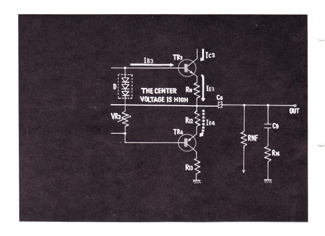
54. WHEN THE RESISTOR R<sub>12</sub> IS OPEN, THE EMITTER CURRENT OF TRANSISTOR 4 BECOMES ZERO.
