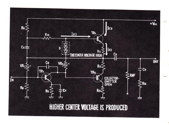
36. IN THIS CASE, NO CURRENT FLOWS BETWEEN THE COLLECTOR AND EMITTER, AND SINCE THE BIAS VOLTAGE IS APPLIED TO TRANSISTOR 3, A HIGH VOLTAGE APPEARS AT THE CENTER POINT.
