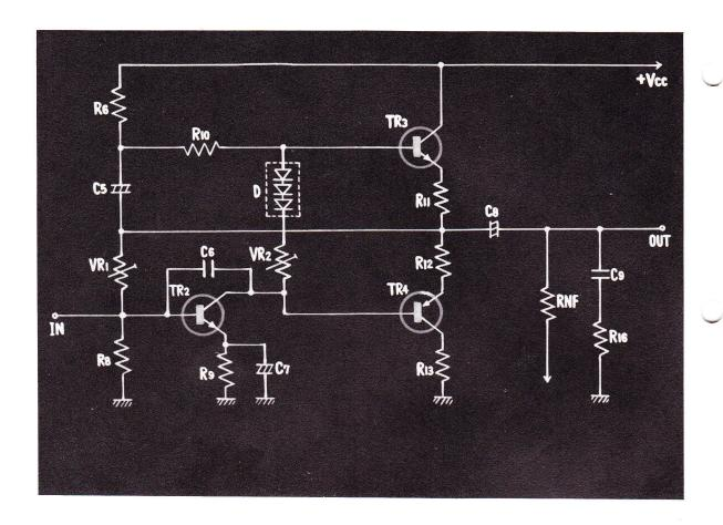
8. SINCE THERE IS NO DIFFERENCE, AT LEAST THE DC FUNCTION IS CONCERNED, WHETHER TRANSISTORS 5 AND 6 ARE CONNECTED OR NOT, LET'S PROCEED WITH OUR SLIDE STUDIES WITH TRANSISTORS 5 AND 6 DISCONNECTED.
