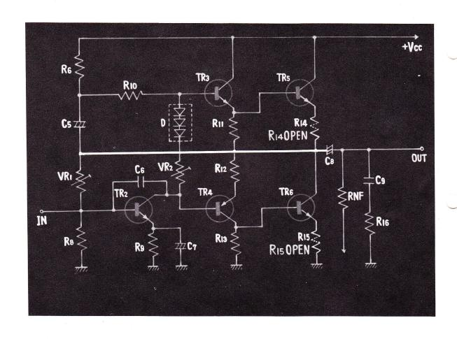
$^{62.}$  WHAT WILL HAPPEN WHEN THE PROTECTIVE RESISTOR  $\text{R}_{\text{14}}$  OR  $\text{R}_{\text{15}}$  FOR TRANSISTORS 5 OR 6 BECOMES OPEN?
