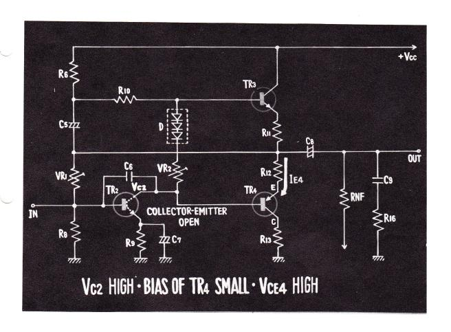
WHEN THE COLLECTOR AND THE EMITTER IS OPEN, THE COLLEC-TOR VOLTAGE OF TRANSISTOR 2 GETS HIGHER. AS A RESULT, THE BIAS FOR TRANSISTOR 4 BECOMES SMALL AND THE VOLTAGE BE-TWEEN THE COLLECTOR AND THE EMITTER RISES.
