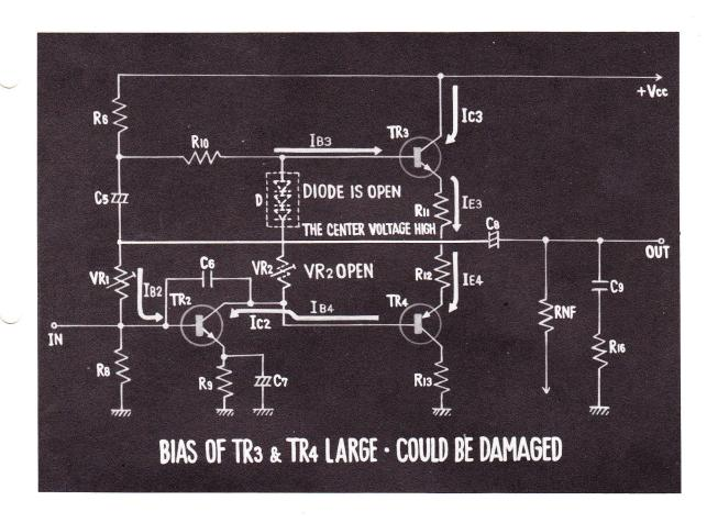
41. HOWEVER, SINCE THE BIAS VOLTAGE IS APPLIED TO TRANSISTOR 2,
