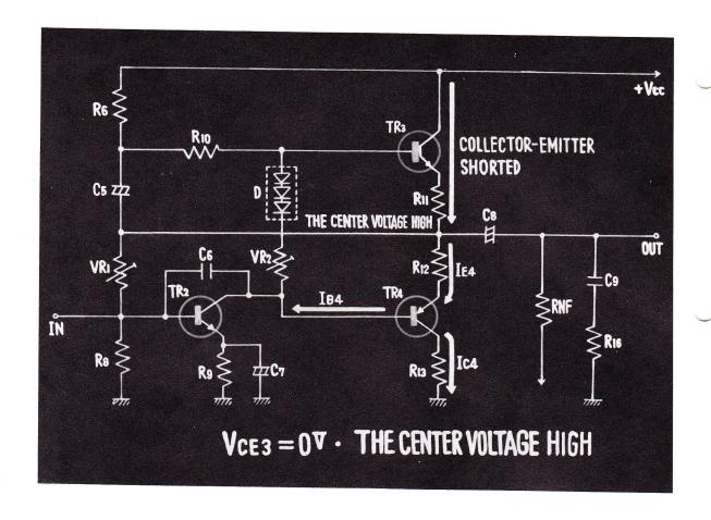
28. WHEN THE COLLECTOR AND THE EMITTER OF TRANSISTOR 3 BECOME SHORTED, THE VOLTAGE BETWEEN THE COLLECTOR AND THE EMITTER BECOMES ZERO (OV), AND AS CURRENT FLOWS DIRECTLY TO THE CENTER POINT FROM VCC THROUGH R11, THE VOLTAGE AT THE CENTER POINT BECOMES HIGHER. IN THIS CASE, THE BIAS FOR TRANSISTOR 4 BECOMES LARGER, CAUSING AN INCREASE IN THE COLLECTOR CURRENT, THEREFORE, EVERY CAUTION IS NECESSARY TO PREVENT TRANSISTOR 4 FROM BEING DAMAGED.
