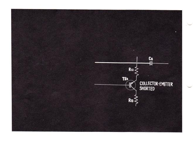
32. WHAT IF THE COLLECTOR AND THE EMITTER OF TRANSISTOR 4 ARE SHORTED?
