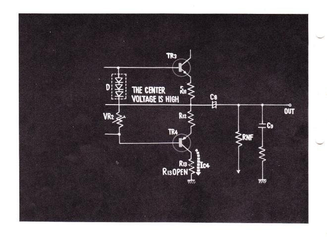
58. WHEN THE RESISTOR R<sub>13</sub> IS OPEN AND ALSO IF TRANSISTOR 6 IS NOT CONNECTED, THEN THE COLLECTOR CURRENT OF TRANSISTOR 4 BECOMES ZERO. AS A RESULT, THE CENTER VOLTAGE WILL GET HIGHER.
