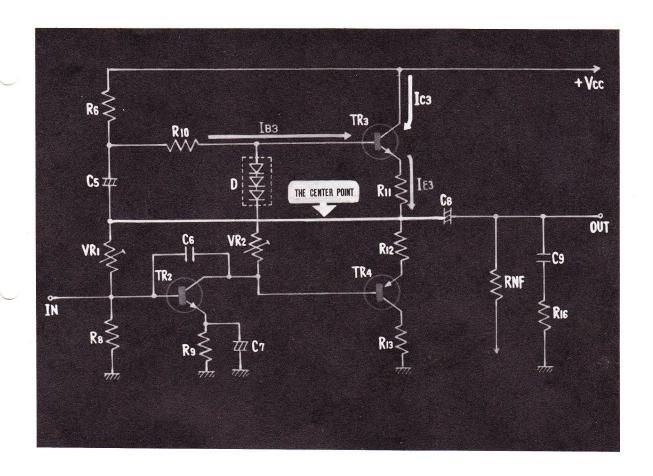
9. NOW LET'S CONSIDER THE DIRECT CURRENT FUNCTION OF THIS CIRCUIT. IF  $V_{C\,C}$  IS APPLIED, A BIAS VOLTAGE IS GIVEN TO TRANSISTOR 3 BY MEANS OF THE RESISTORS  $R_6$  AND  $R_{10}$ . THEN THE COLLECTOR CURRENT OF TRANSISTOR 3, OR  $I_{C\,3}$ , FLOWS, AND A VOLTAGE ARISES AT THE CENTER POINT.
