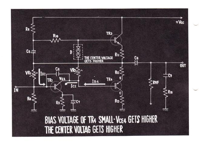
16. FOR THIS REASON, THE BIAS VOLTAGE FOR TRANSISTOR 4 BECOMES SMALLER, AND THE VOLTAGE DROP BETWEEN THE COLLECTOR AND THE EMITTER BECOMES LARGER WHICH TENDS TO RAISE THE CENTER VOLTAGE.
