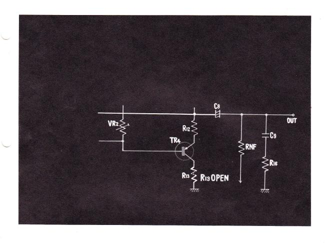
57. NEXT, WHAT ABOUT THE CASE WHEN THE RESISTOR  $R_{13}$  IS OPEN?
