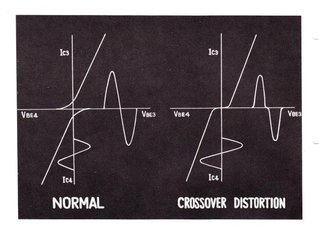
38. WHEN THE DIODE IS SHORTED, THE BIAS VOLTAGE IN THE DRIVE-STAGE AND POWER-STAGE BECOMES SMALL, CAUSING THE FUNCTION POINT SHIFT ONTO THE NON-LINEAR PORTION OF THE  $V_{\rm B}$  I<sub>C</sub> CHARACTERISTIC.
