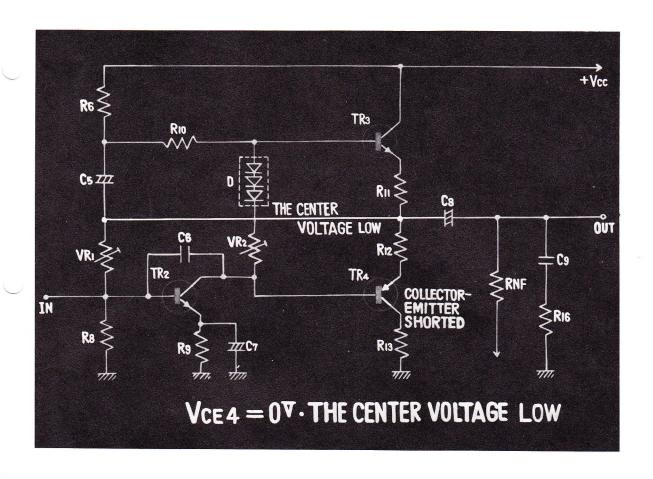
WHEN THE COLLECTOR AND THE EMITTER ARE SHORTED, THE VOLTAGE BETWEEN THE COLLECTOR AND THE EMITTER OF TRANSISTOR 4 BECOMES OV AND THE VOLTAGE AT THE CENTER POINT GETS LOWER.
