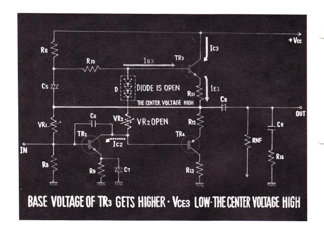
40. IN THIS CASE, THE COLLECTOR CURRENT OF TRANSISTOR 2 DOES NOT FLOW. THEREFORE, AS THE BASE VOLTAGE OF TRANSISTOR 3 INCREASES, THE BIAS VOLTAGE OF TRANSISTOR 3 GETS LARGER. CONSEQUENTLY THE VOLTAGE BETWEEN THE COLLECTOR AND EMITTER BECOMES LOWER, AND THE VOLTAGE AT THE CENTER POINT BECOMES HIGHER THAN  $1/2\ V_{CC}$ .
