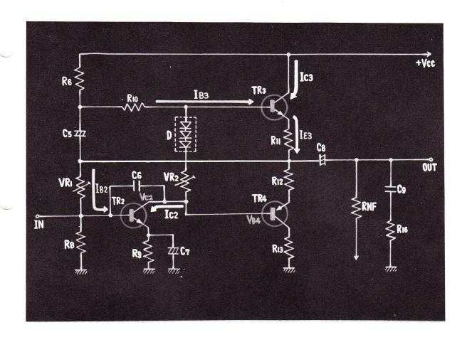
THE COLLECTOR OF TRANSISTOR 2 IS DIRECTLY CONNECTED TO THE BASE OF TRANSISTOR 4 SO THAT THE BASE VOLTAGE, OR  $V_{B\,4}$ , OF TRANSISTOR 4 ALSO DROPS.
