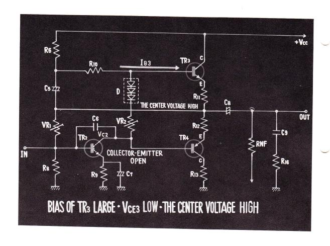
26. ON THE OTHER HAND, THE BIAS IN TRANSISTOR 3 BECOMES LARGER, AND THE VOLTAGE BETWEEN THE COLLECTOR AND THE EMITTER DROPS. AND THE CENTER VOLTAGE BECOMES HIGHER THAN THE NORMAL VALUE OF  $1/2\ V_{CC}$ .
