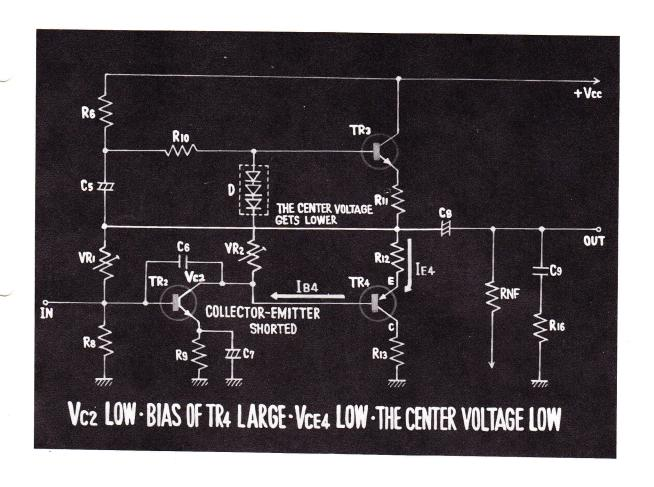
WHEN THE COLLECTOR AND THE EMITTER OF TRANSISTOR 2 ARE SHORTED, THE COLLECTOR VOLTAGE OF TRANSISTOR 2 BECOMES LOW, THUS THE BIAS VOLTAGE OF TRANSISTOR 4 BECOMES LARGER. THEN, THE VOLTAGE DROP BETWEEN THE COLLECTOR AND THE EMITTER OF TRANSISTOR 4 GETS SMALLER. THEREFORE, THE CENTER VOLTAGE ALSO GETS LOWER.
