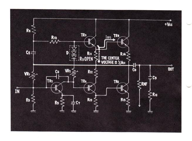
52. HOWEVER, IN ACTUAL CIRCUITS, TRANSISTOR 5 IS ALWAYS CONNECTED. THEREFORE, THE EMITTER VOLTAGE OF TRANSISTOR 3 BECOMES THE BASE CURRENT OF TRANSISTOR 5, MAINTAINING THE CENTER VOLTAGE AT  $1/2\ V_{CC}$  OF THE NORMAL VALUE.
