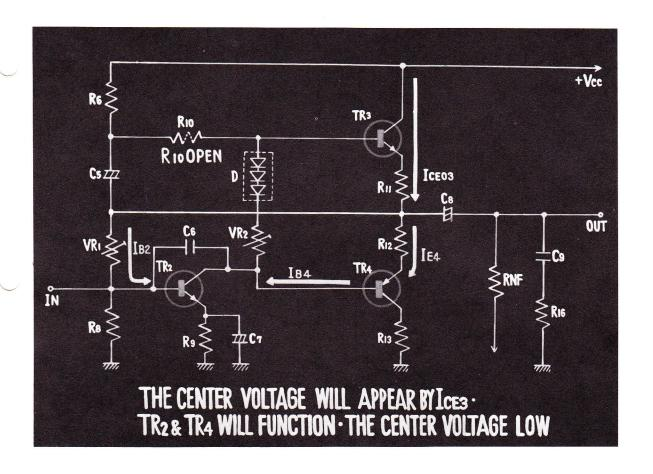
49. IN THIS CASE, IT MAY SEEM THAT NO VOLTAGE IS PRODUCED AT THE CENTER POINT SINCE NO BIAS VOLTAGE IS APPLIED TO TRANSISTOR
