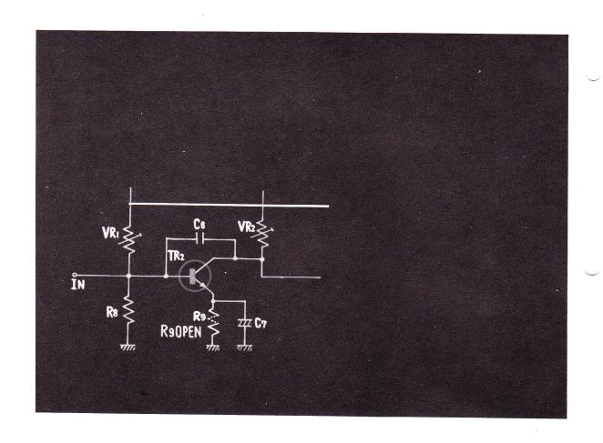
46. WHAT ABOUT THE CASE WHEN THE RESISTOR  $R_{\rm 9}\,$  IS OPEN?
