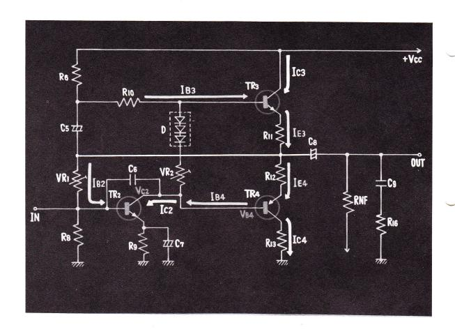
12. SINCE TRANSISTOR 4 IS A P-N-P TYPE, A BIAS VOLTAGE IS IN FACT GIVEN TO TRANSISTOR 4, AND CURRENT THUS FLOWS TO TRANSISTOR 4.
