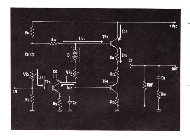
10. A BIAS VOLTAGE IS GIVEN TO TRANSISTOR 2 FROM THE CENTER POINT THROUGH  $VR_1$  WHICH IS FOR REGULATING THE CENTER VOLTAGE. THEN THE COLLECTOR CURRENT FOR TRANSISTOR 2, OR  $I_{C\,2}$ , STARTS TO FLOW, AND THE COLLECTOR VOLTAGE, OR  $V_{C\,2}$ , DROPS.
