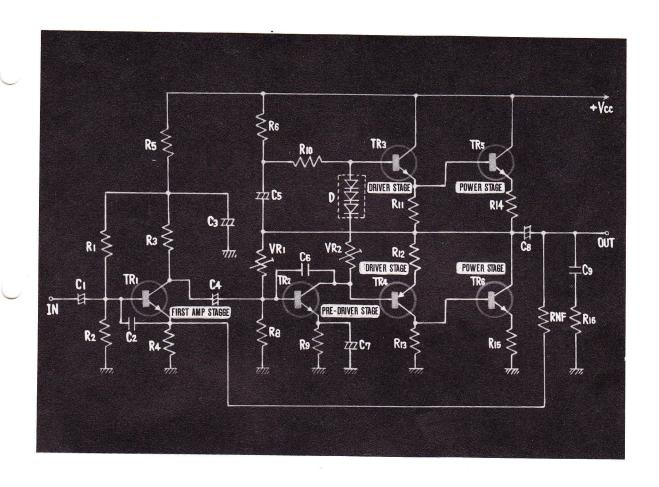
ON THIS BASIC DIAGRAM, TRANSISTOR 1 IS FOR THE PRIMARYSTAGE AMPLIFICATION, TRANSISTOR 2 IS FOR THE PRE-DRIVING
