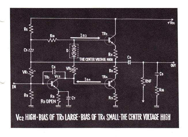
47. IN THIS CASE, NO CURRENT FLOWS INTO TRANSISTOR 2, MAKING ITS COLLECTOR VOLTAGE HIGHER. THE BIAS VOLTAGE OF TRANSISTOR 3 BECOMES LARGER, WHILE THAT OF TRANSISTOR 4 BECOMES SMALLER, AND AS A RESULT THE CENTER VOLTAGE BECOMES HIGHER THAN  $1/2\ V_{CC}$ .
