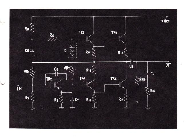
65. IN THIS INSTANCE, REMOVE THE POWER TRANSISTORS AND CHECK IF THE CENTER VOLTAGE IS SET AT  $1/2\ V_{CC}$ . IF THE VOLTAGE IS NORMAL, THEN INSTALL A NEW POWER TRANSISTOR.
