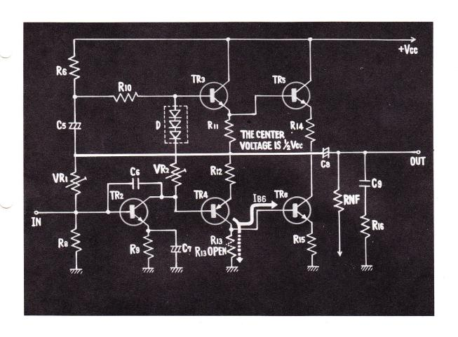
$^{59.}$  IF TRANSISTOR 6 IS CONNECTED IN THE CIRCUIT, THE COLLECTOR CURRENT OF TRANSISTOR 4 BECOMES THE BASE CURRENT OF TRANSISTOR 6, MAINTAINING THE CENTER VOLTAGE AT 1/2  $V_{\text{CC}}$  OR THE NORMAL VALUE.
