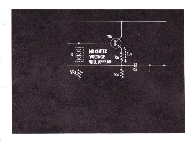
$^{51}$ . WHEN THE RESISTOR  $R_{11}$  IS OPEN IN THIS CIRCUIT WHERE TRANSISTOR  $^{5}$  IS NOT CONNECTED, THE CENTER VOLTAGE WILL NOT APPEAR.
