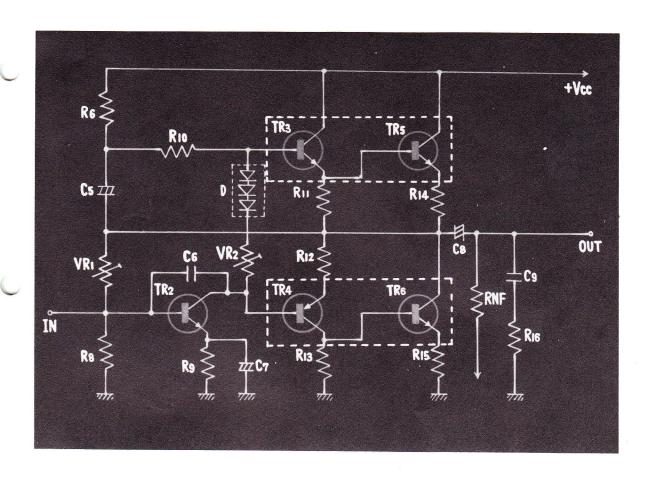
7. TRANSISTORS 3 AND 5 AS WELL AS TRANSISTORS 4 AND 6 ARE OF DARLINGTON-CONNECTION, SO THAT THEY MAY BE CONSIDERED AS N-P-N AND P-N-P TRANSISTORS, RESPECTIVELY.
