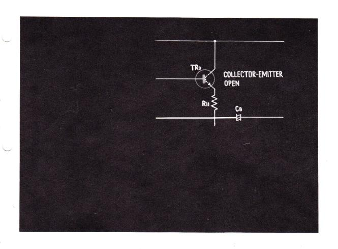
29. WHAT IF THE COLLECTOR AND THE EMITTER OF TRANSISTOR 3 IS OPEN?
