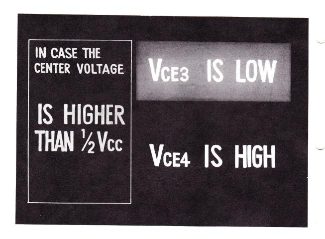
20. WHEN THE CENTER VOLTAGE IS HIGHER THAN 1/2  $V_{CC}$ , IT MAY BE THAT THE VOLTAGE BETWEEN THE COLLECTOR AND THE EMITTER OF TRANSISTOR 3, OR  $V_{CE3}$ , IS LOW, OR, ON THE CONTRARY, IT MAY BE THAT THE VOLTAGE BETWEEN THE COLLECTOR AND THE EMITTER OF TRANSISTOR 4, OR  $V_{CE4}$ , IS HIGH.
