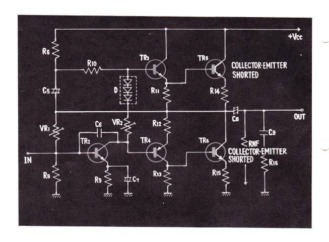
64. HOW ABOUT THE CASE WHEN POWER TRANSISTOR 5 OR 6 IS SHORT-ED? WHEN EITHER ONE OF THE POWER TRANSISTORS IS SHORTED, THE FUSE WILL BLOW IMMEDIATELY, MAKING IT IMPOSSIBLE TO CHECK THE CONDITION BY MEANS OF VOLTAGE.
