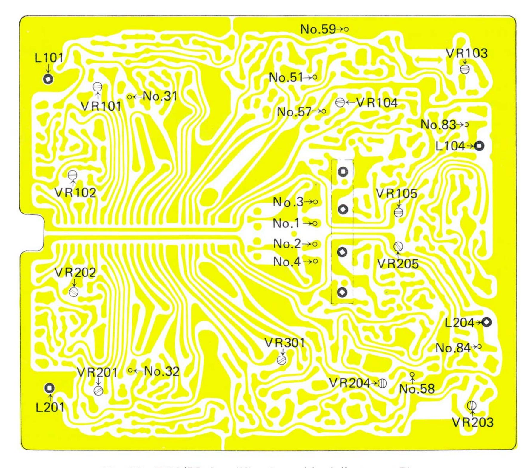
Fig. 29 REC/PB Amplifier Assembly Adjustment Places
