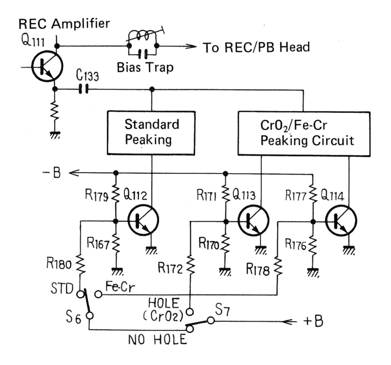
Fig. 7 Recording Equalizer Changeover Circuit
