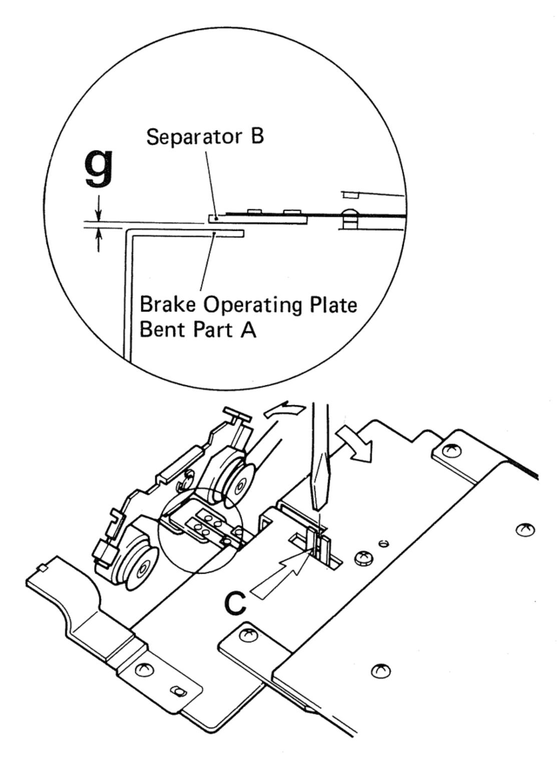
Fig. 23 Adjustment of the Motor Switch -
