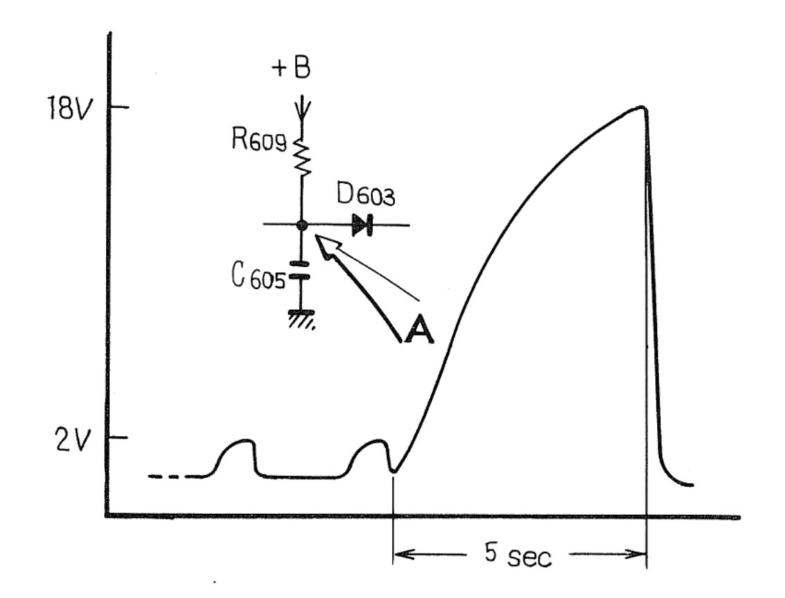
Fig. 10 The Potential at Point A
