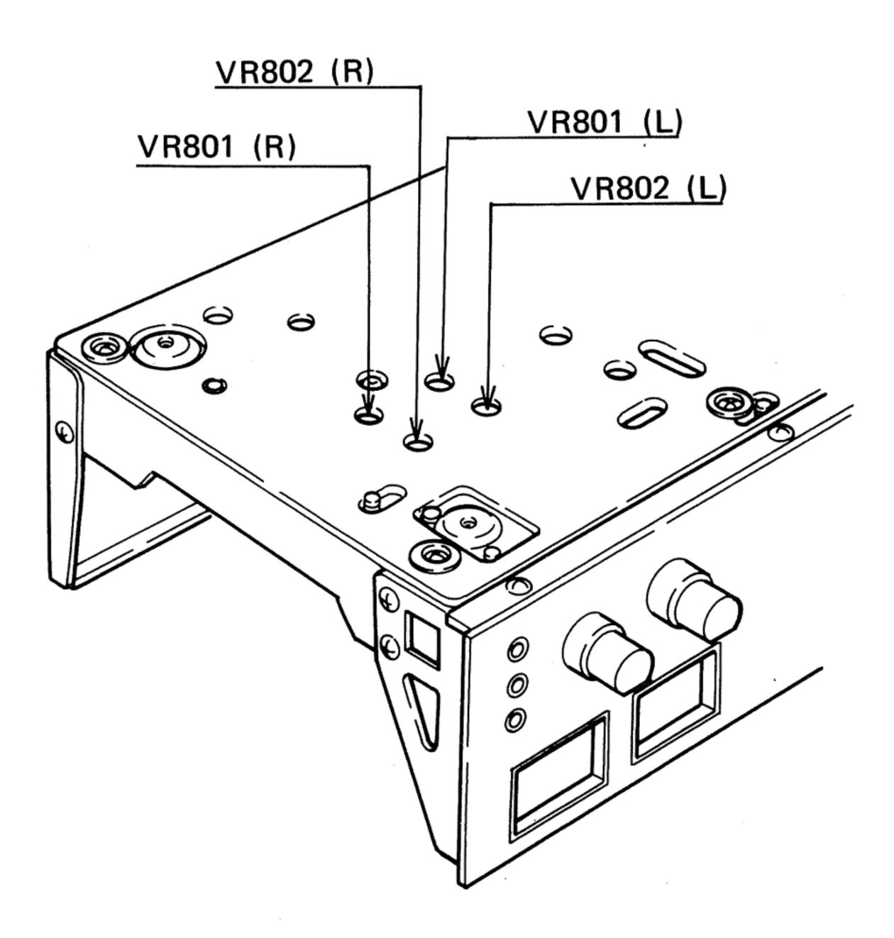
Fig. 34 DOLBY Circuit Adjustment
