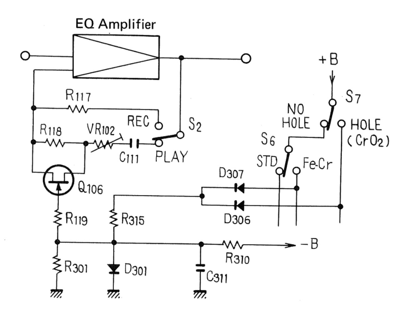
Fig. 6 Playback Equalizer Changeover Circuit
