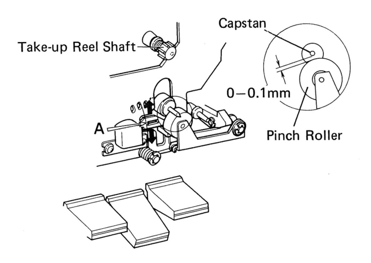
Fig. 21 PLAY Timing Adjustment
