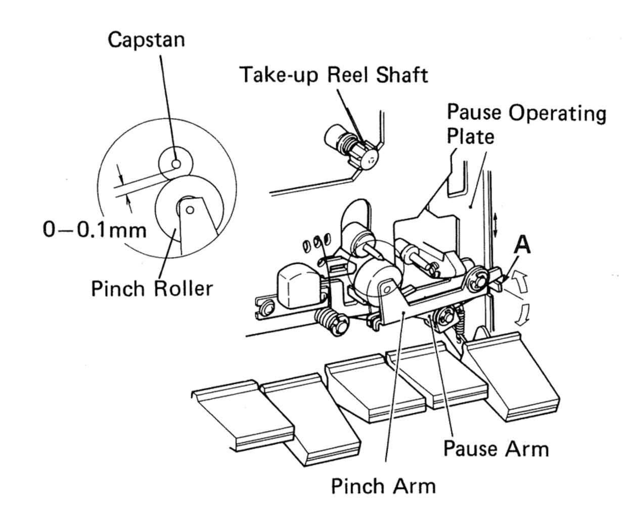
Fig. 22 PAUSE Timing Adjustment
