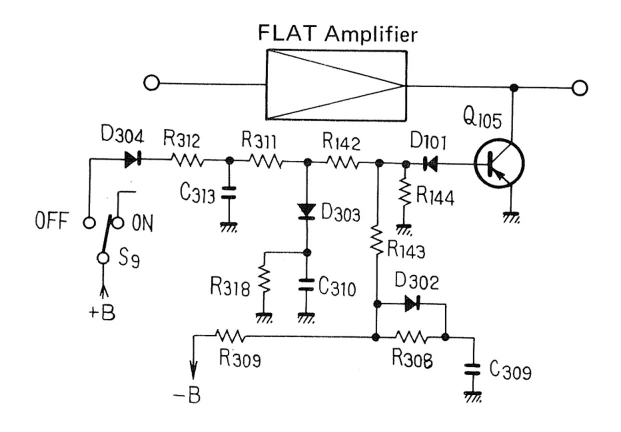
Fig. 8 Muting Control Circuit
