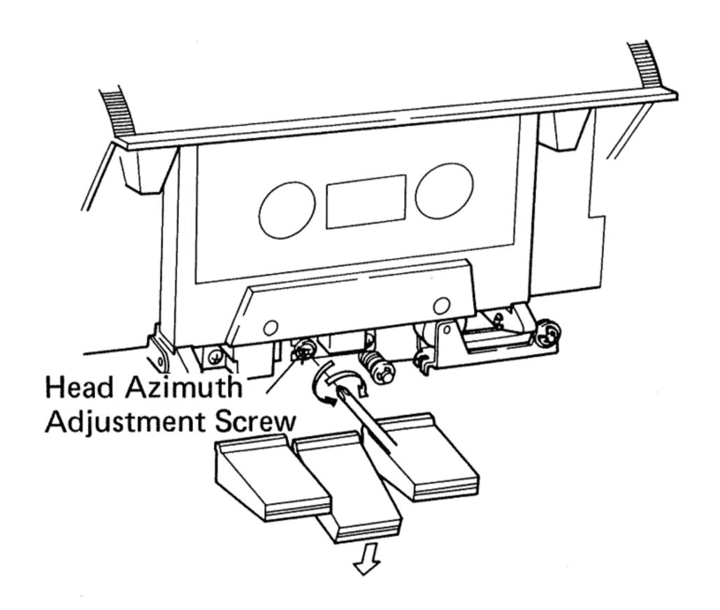
Fig. 27 Head Azimuth Adjustment
