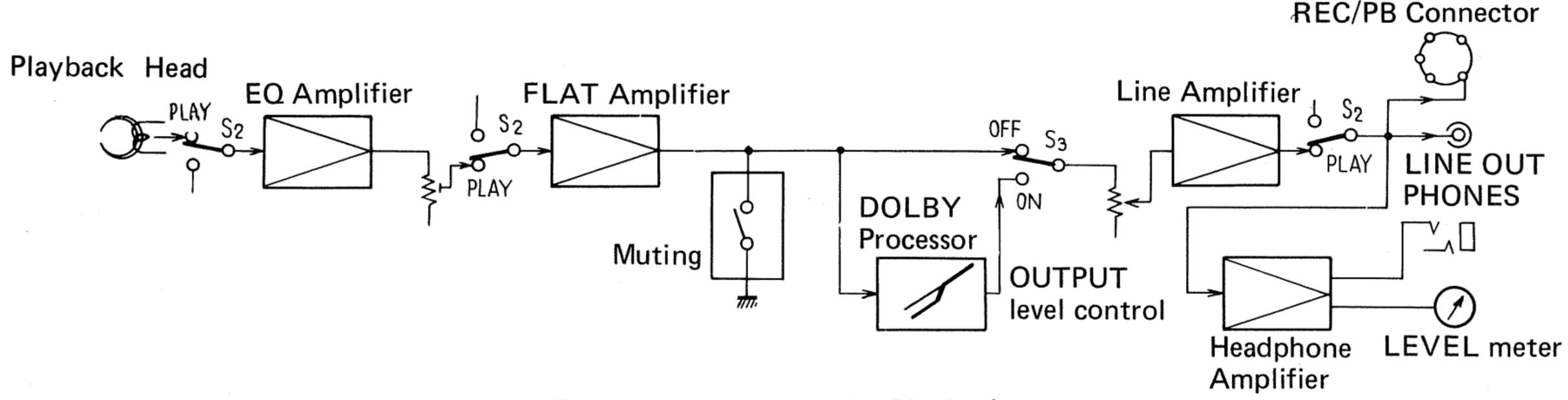
Fig. 1 Signal Path during Playback
