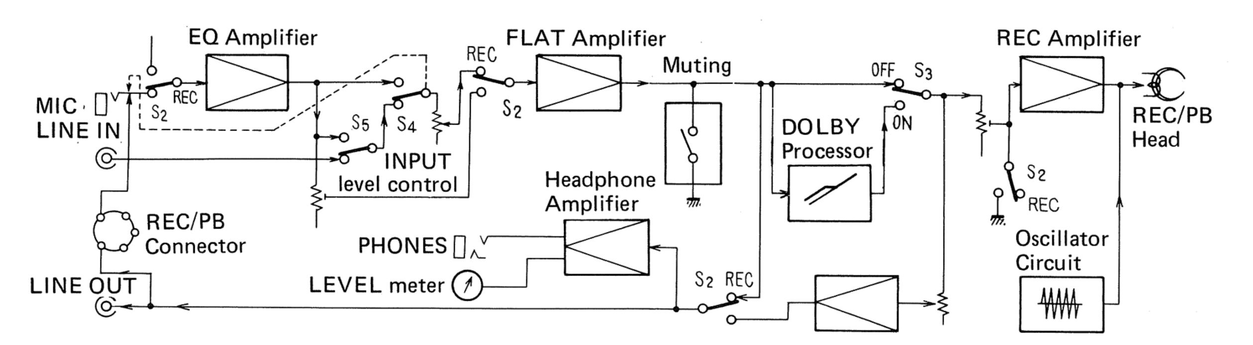
Fig. 2 Signal Path during Recording
