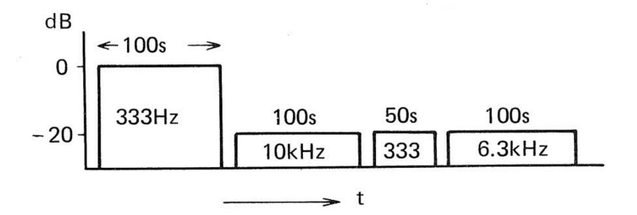
Fig. 25 Recorded Contents of Tape STD-341
