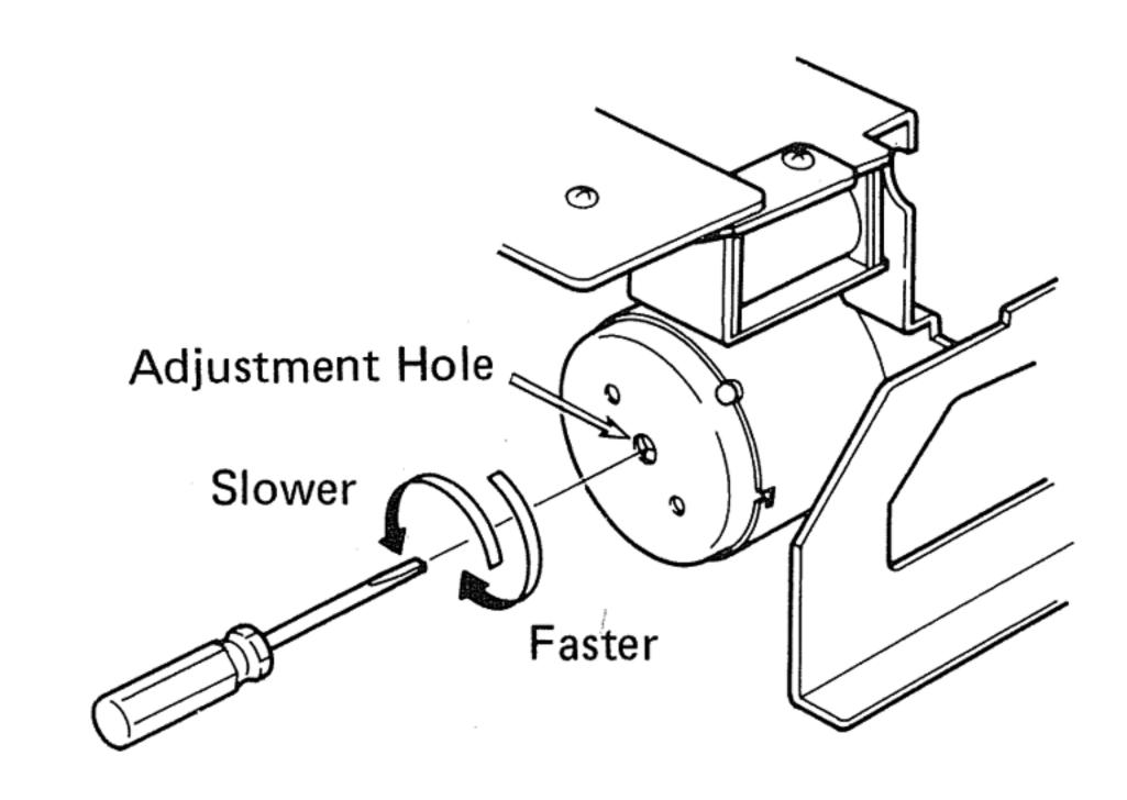
Fig. 20 Adjustment of Tape Transport
