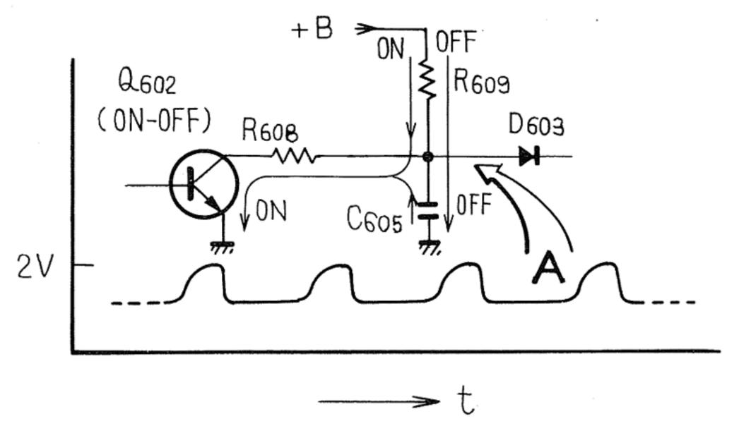
Fig. 9 The Potential at Point A
