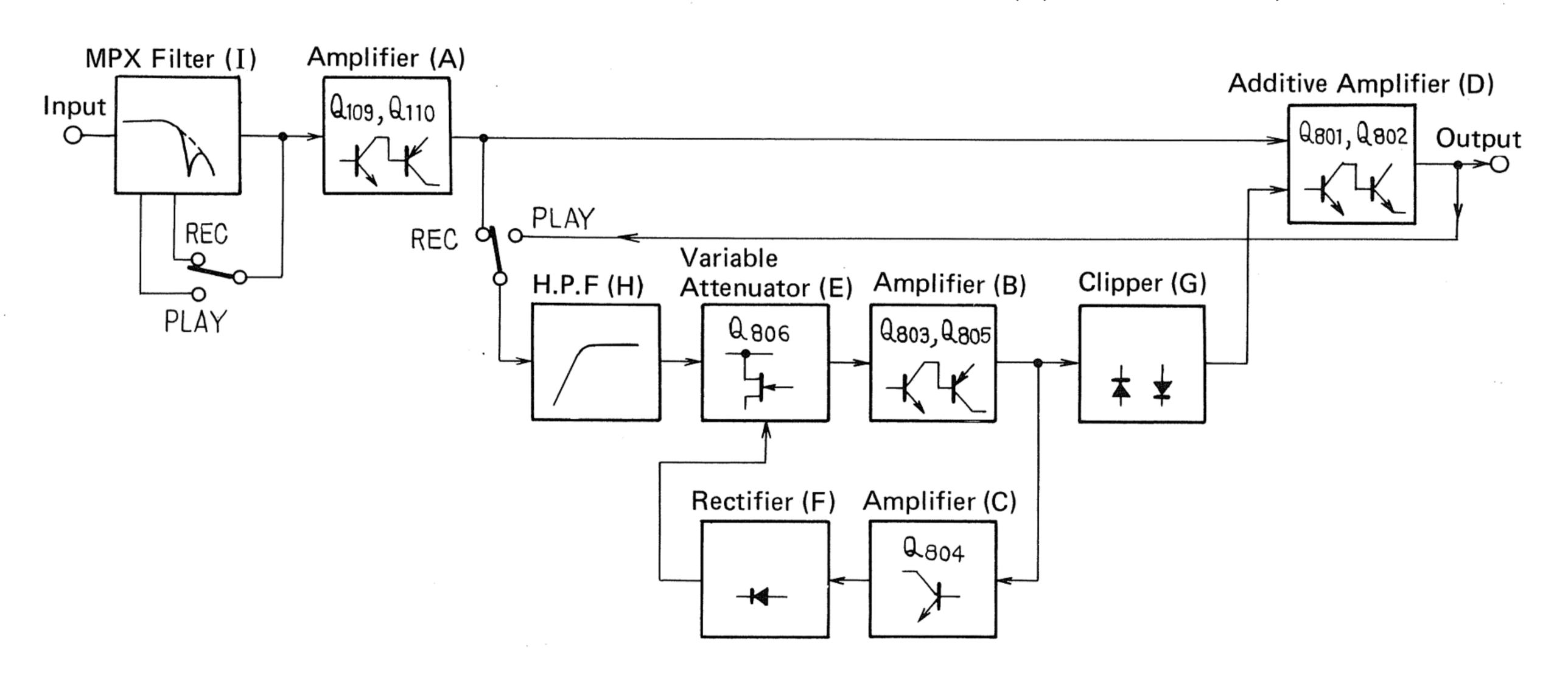
Fig. 3 Configuration of the DOLBY Processor
