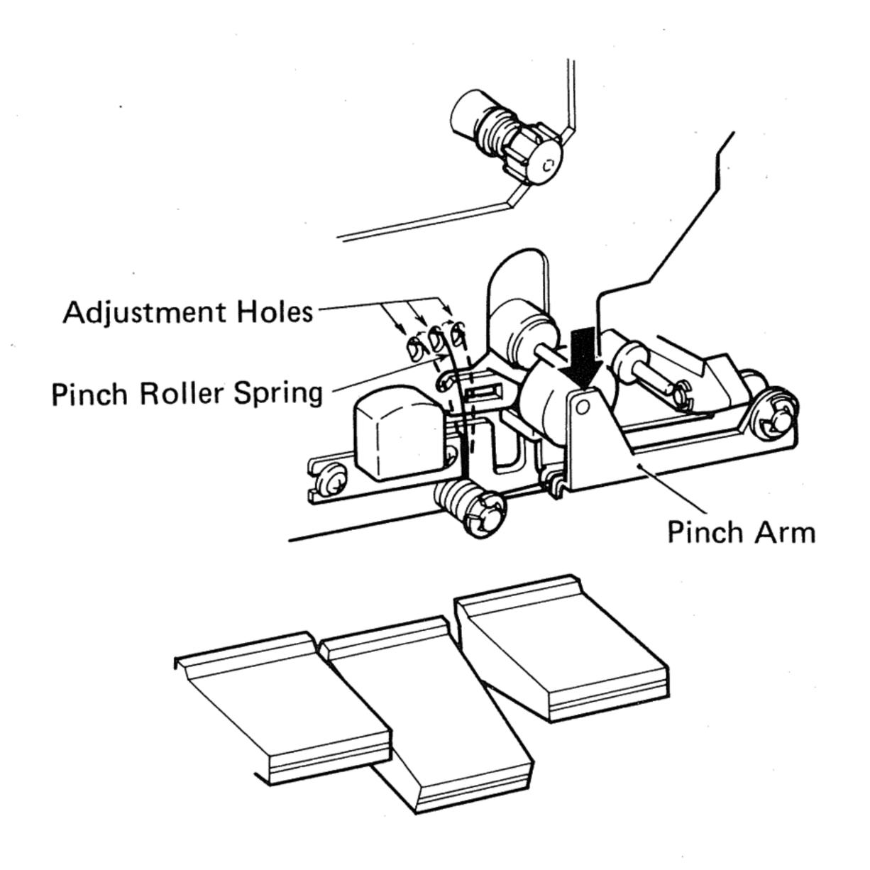
Fig. 19 Adjustment of Pinch Roller Pressure
