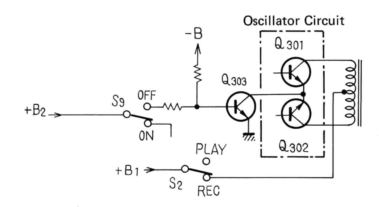
Fig. 4 Operational Control of the Oscillator Circuit
