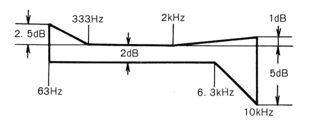
Fig. 28 Playback Frequency Response (Using STD-331, and the STD Position, with DOLBY NR OFF
