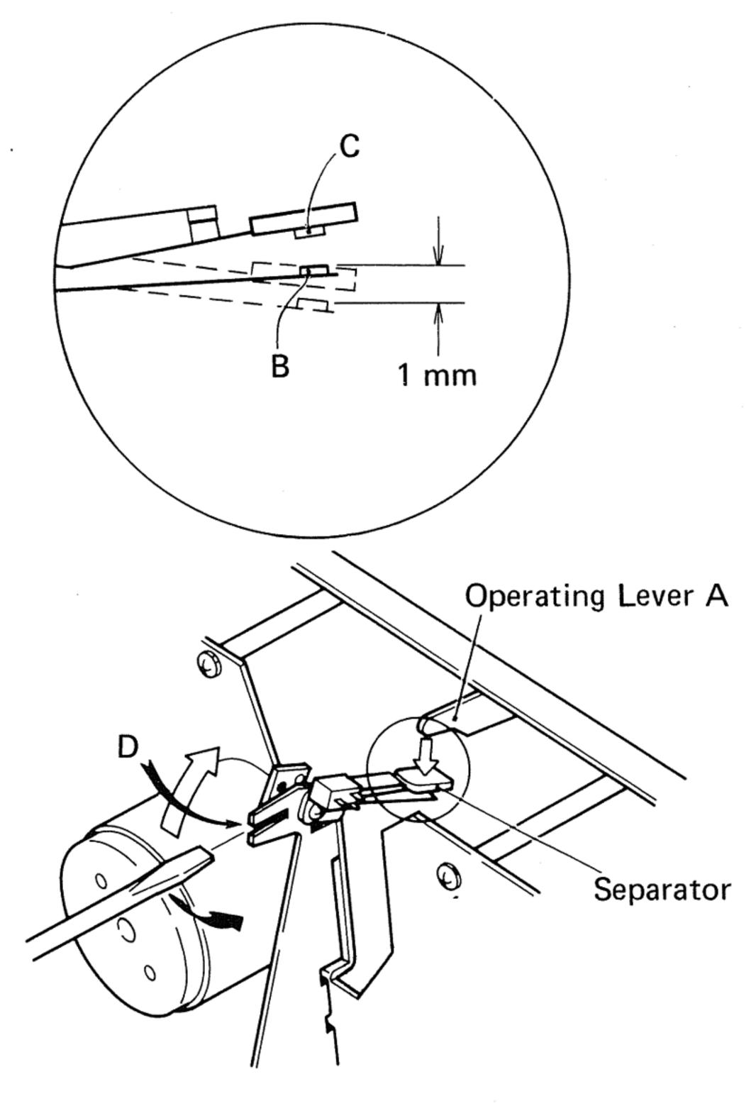
Fig. 24 Muting Switch Adjustment
