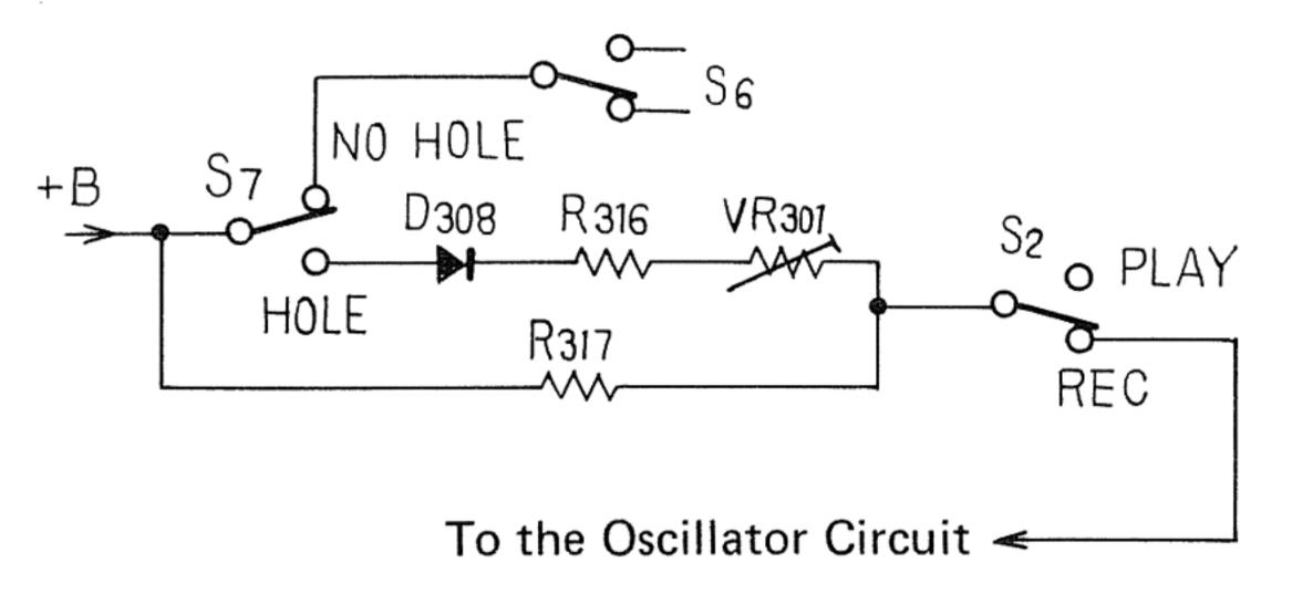
Fig. 5 Recording Bias Changeover Circuit
