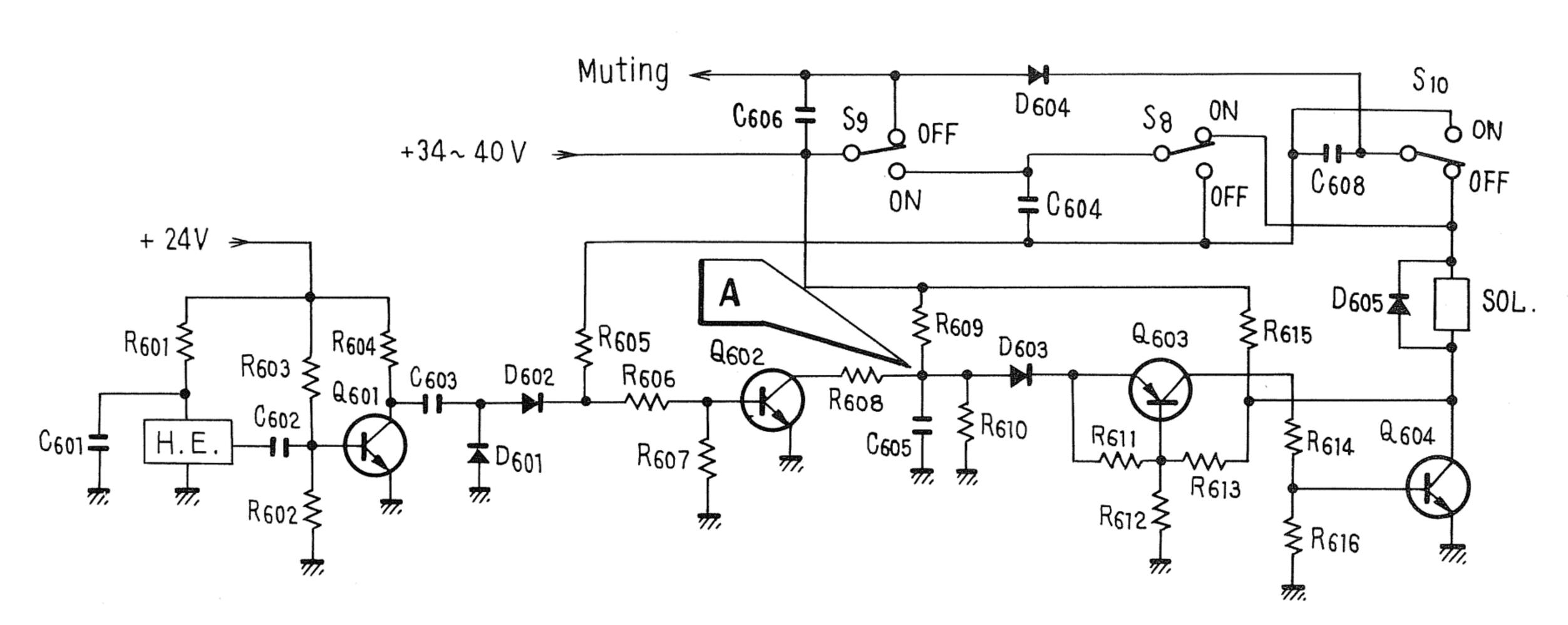
Fig. 11 Schematic Diagram of Auto Stop Circuit
