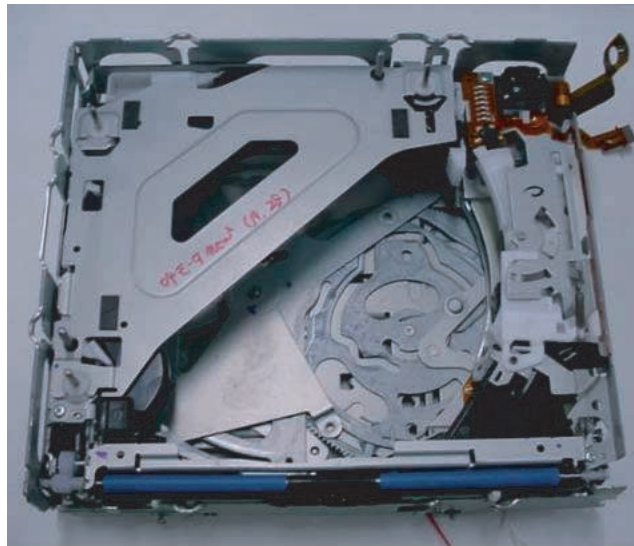
The STG unit is properly assembled
