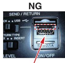
The USB connector is not placed properly in the opening of the USB panel.
