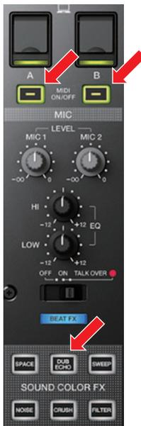
You can turn the unit on even during a shutoff of the secondary power triggered by a voltage error, by entering Error Detection OFF mode. To enter this mode, while holding the MIDI ON/OFF buttons and SOUND COLOR FX (DUB ECHO) button pressed simultaneously, press the POWER button (to set it to ON).
