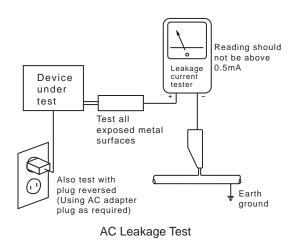
ANY MEASUREMENT NOT WITHIN THE LIMITS OUTLINED ABOVE ARE INDICATIVE OF A POTENTIAL SHOCK HAZARD AND MUST BE CORRECTED BEFORE RERTURNING THE APPLIANCE TO THE CUSTOMER.
