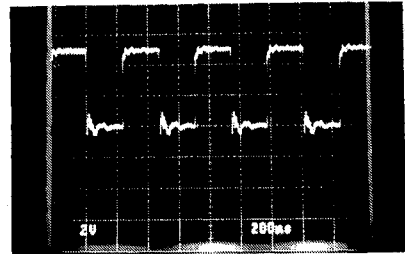
⑬ IC3-79 Pin : STOP MODE 2V/div 5μsec/div
