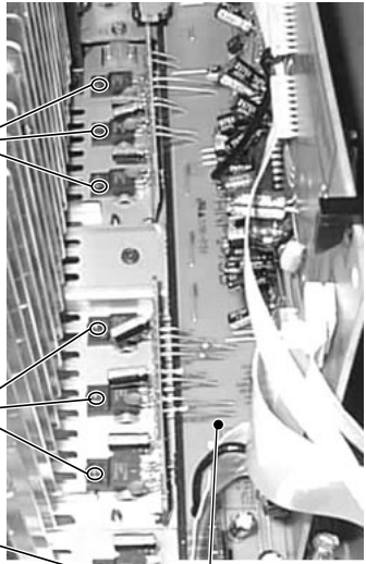
REGULATOR Assy Replace the Regulator IC.
