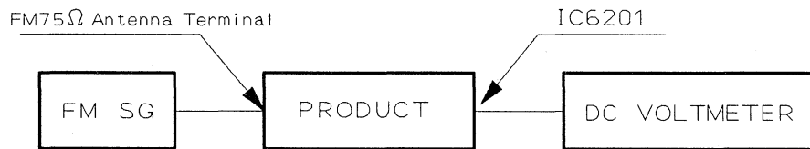
Fig. 1 FM Adjustment Connection Diagram
