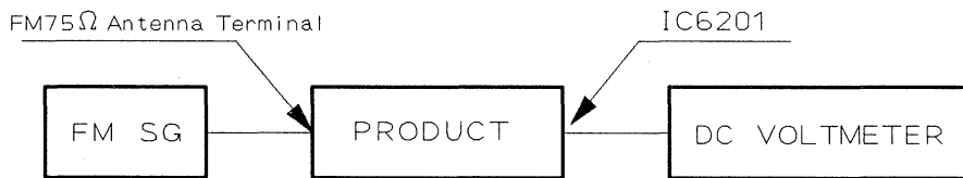
Fig. 1 FM Adjustment Connection Diagram
