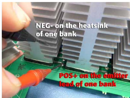
Figure 5.2 - Quick output transistor check (Ch2-)
