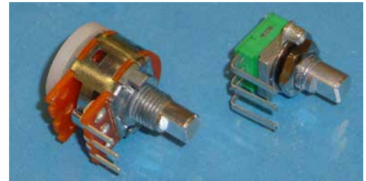
Figure 5.7 - New sealed gain pot (on the right)
