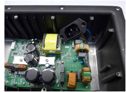
Figure 9.2 - Powering up just the PSU/amp board
