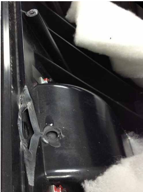
Figure 9.16 - Broken enclosure - this speaker is not repairable.
