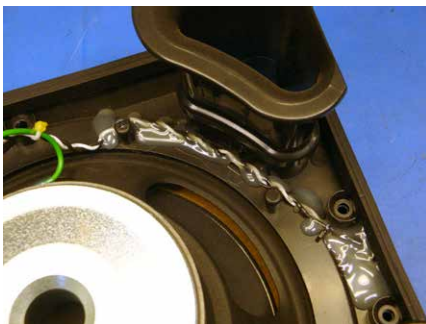
Figure 9.12 - Front LED wire routing
