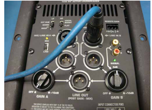
Figure 8.4 - Input connection to Ch.B
