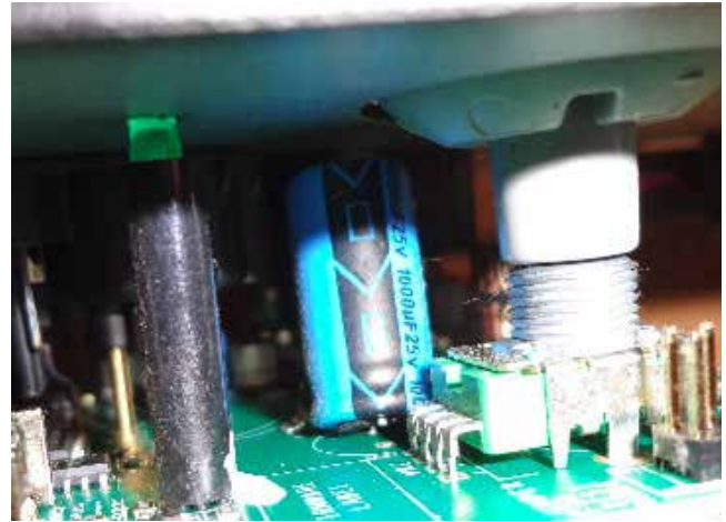
Figure 9.7 - Broken capacitor C45
