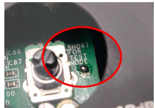
Figure 8.3 - Test mode activated
