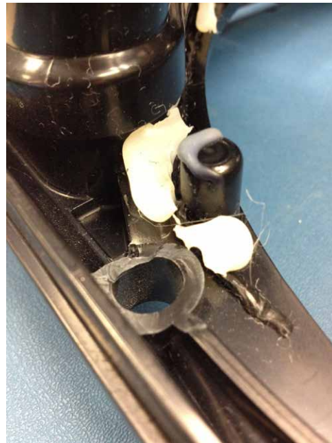
Figure 9.17 - Broken baffle near screw mounting hole. New baffle assemblies are available.
