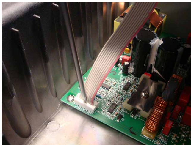
Figure 7.2 - Put pressure on the white housing to release the ribbon cable
