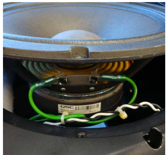
Figure 9.10 - One of these fastons can disconnect easily from the LF transducer's terminals
