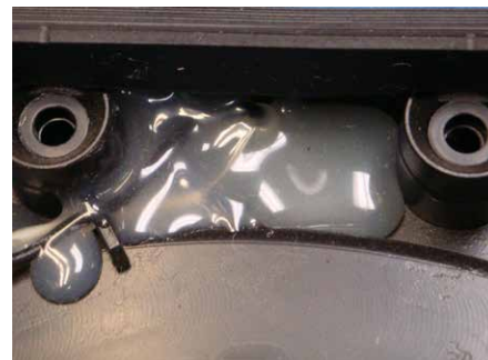
Figure 9.13 - Glue covering the front LED
