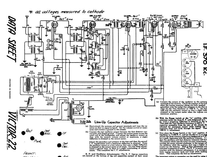
The important points to remember are the need for using t oscillator output to obtain a deflection in the output meter wite control at its maximum position and the manner of obtainin high frequency oscillator and detector adjustments.
