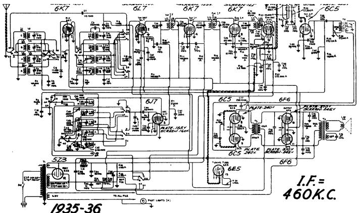
I-F Adjustments—Connect the output of the test Oscillator from the Type-6L7 first detector control grid to chassis-ground and adjust its frequency to 460 kc. Tune the receiver to Band "A", setting the station selector at a point where no interference is received from local stations or the local oscillator. Then tune the i-f trimmers C-31, C-30, C-28, C-27, C-24 and C-23 in order, each for maximum indicated receiver output.
