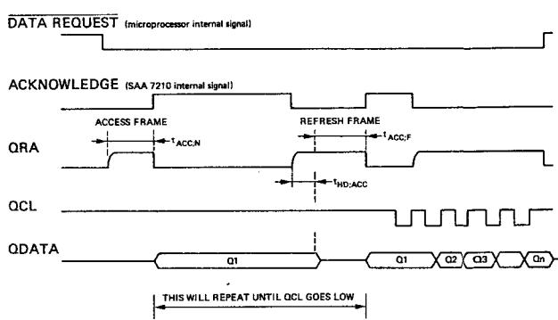
Fig. 4.4.2 Q-CHANNEL TIMING WAVEFORMS (refresh mode)
