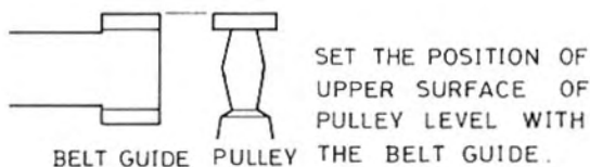
Fig. 4 Positioning of Pulley
