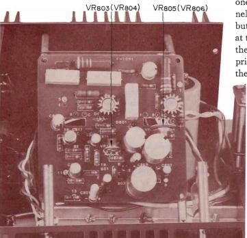
Only the test points for one of the stereo channels are indicated here, but test points also exist at the same positions on the corresponding printed circuit sheet for the other channel.
