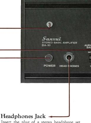
Insert the plug of a stereo headphone set into this jack for private listening. Though any type of headphone set with a plug which matches this jack can be used, a dynamic type stereo headphone set is recommended.
