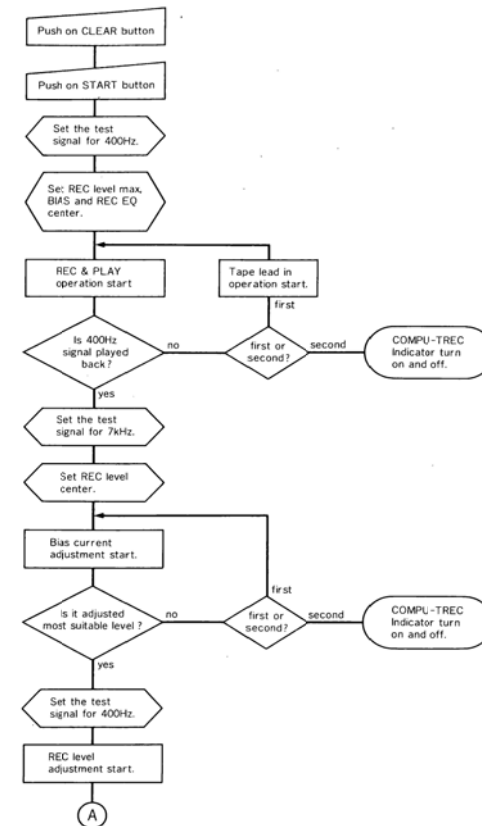
Fig. 2-4 Flow chart of COMPU-TREC operation
