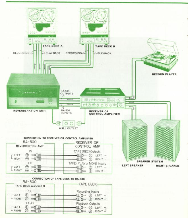
To Reverberate Sound From Any Program Source—Record Player, Tuner or Microphone—Except Tape Deck
