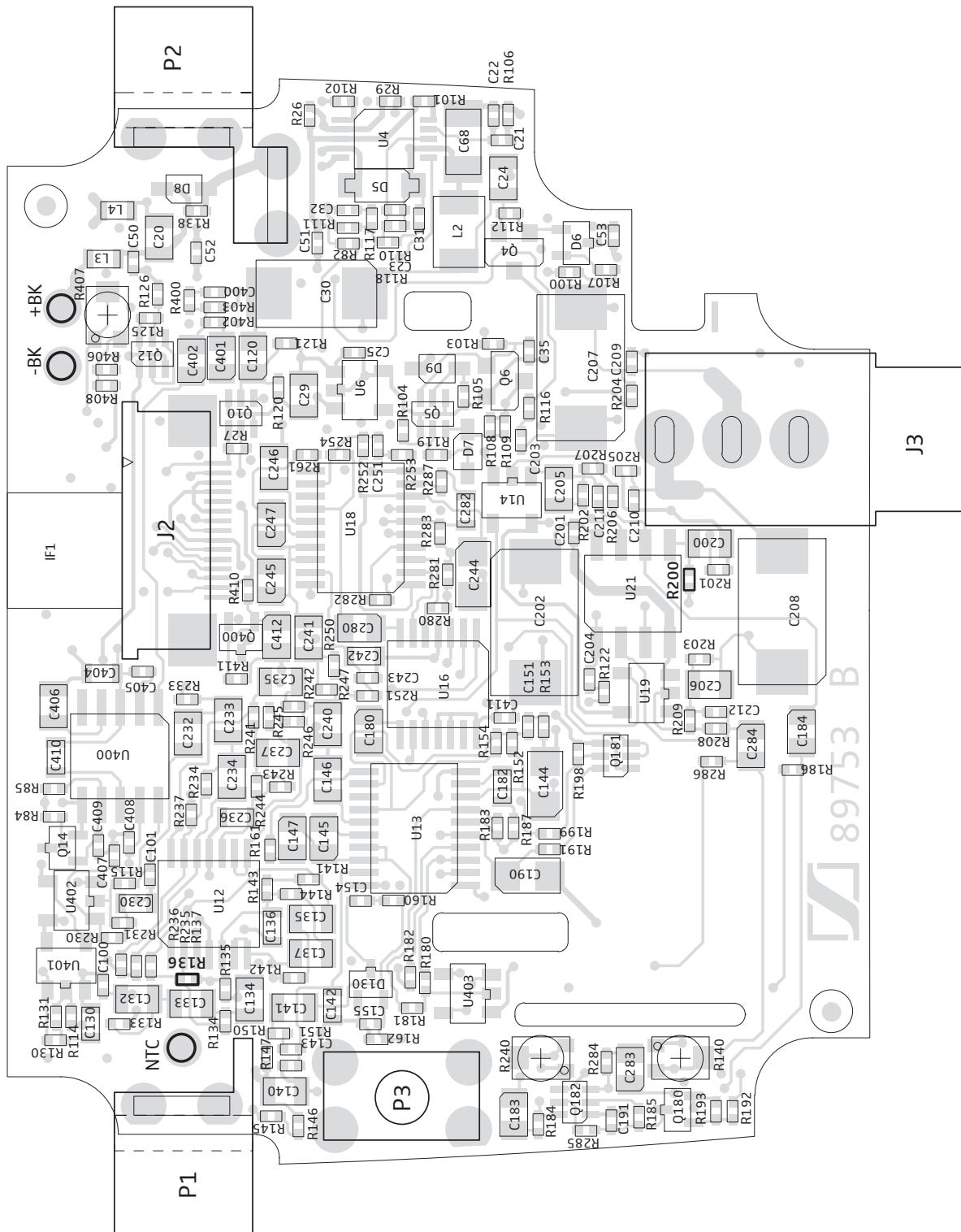
Mainboard, printed circuit board, component side
