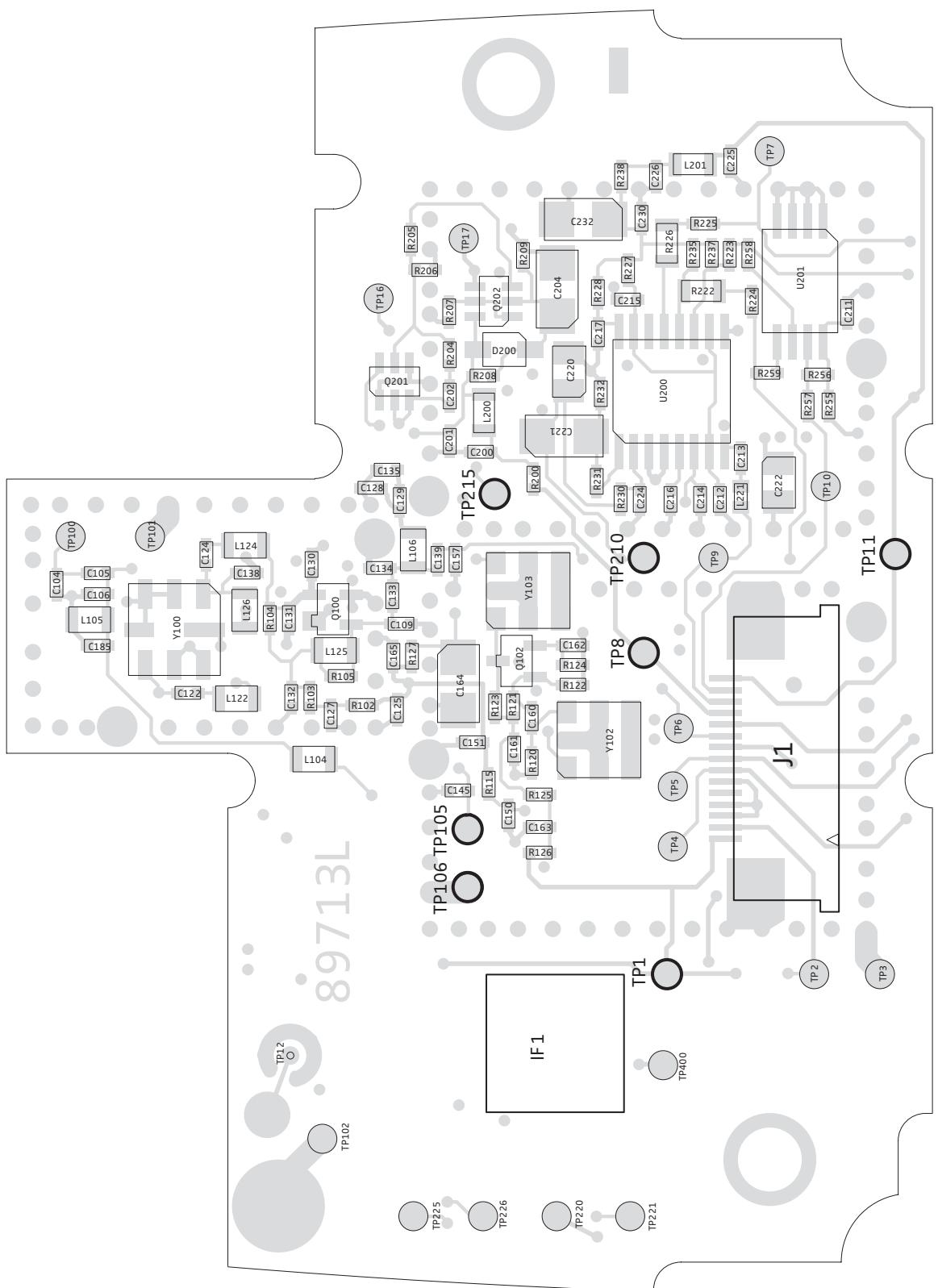
**RF module, printed circuit board, solder side**
