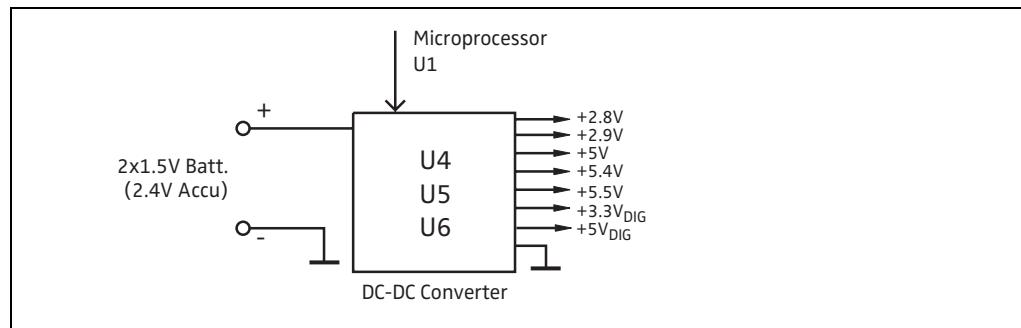
The receiver can be powered by either two batteries or the BA 2015 battery pack. The operating time can be increased via the following partial voltages produced by the U200 DC/DC converter from the rated voltage of 2.4 V<sub>DC</sub>:
