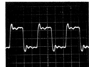
20 IC301 13 pin (128FS) 6.4Vp-p, 0.18μsec
