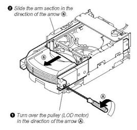
Gently pull out the stocker block that has been moved slightly forward, to reveal the LOADING MOTOR (page 112, M871). Pull out the stocker block as far as possible. Rotate, with your fingers the PULLEY(page 112, 956) around which the loading motor belt is wound, to rotate the stocker by 90 degrees.
