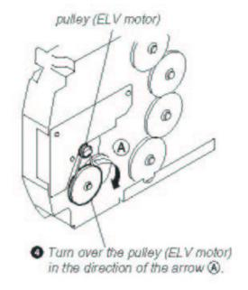
Remove the base (a not-supplied part shown at the bottom of page 114) installed in the CDM80, and rotate the PULLEY (GEAR) (1054 on page 114) clockwise to eject the disc.
