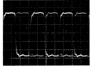
39 IC362 4pin (LRCK) 5.6Vp-p, 0.52μs
