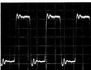
25 IC307 58pin (F128) 5.8Vp-p, 0.17μs
