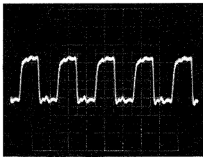
34 IC307 14pin (XT1I) 2.8Vp-p, 18.816MHz
