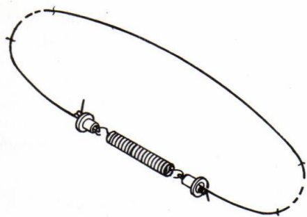
Fig. 2-8 Loop of dial cord
