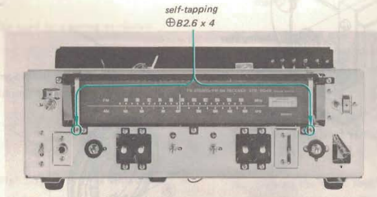
Fig. 2-11 Dial scale replacement
