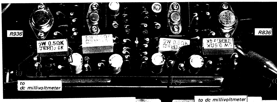
Fig. 3-16 Dc millivoltmeter connection
