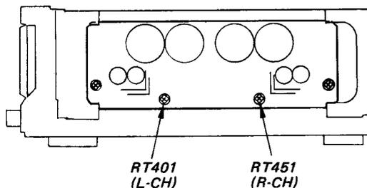
Adjust RT401 (L-CH) and RT451 (R-CH) for 0 V reading on the VOM.
