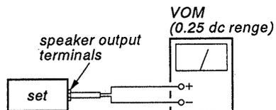
Adjust RT401 (L-CH) and RT-451 (R-CH) for 0 V reading on the VOM.
