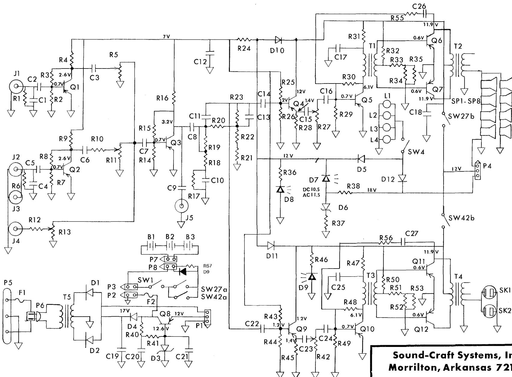
NOTES: All resistors  $\frac{1}{2}$  watt, 10% composition, value in ohms. All capacitors in microfarads. All voltages referenced to (+) positive ground with 20,000 ohms per volt meter. Measurement conditions: Amplifier(s) on. A.C. power connected.
