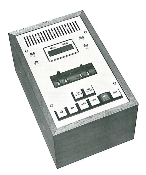
The A80 pre-selection unit enables fast and precise location of a programmed tape position. By simply depressing a push button, the system automatically finds a freely chosen tape timer zero point or predetermined setting. With normally adjusted braking times the locating process takes place without any overshoot.
