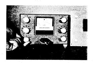
An idling power check discloses the power amplifier is within specs for current consumption, drawing less than 55 watts at 120 volts AC. But the job isn't completed yet!
