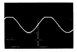
these pots should be readjusted. They control the limiter transistors in the overload protection circuit.
