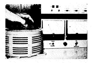
When we measure idling power, we're also checking the speaker protection circuit. The speaker protection relay should energize at a line voltage of about 98 volts AC. This closes the circuit to the speaker output terminals.
