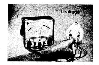
Finally, check the transistor for an emitter to collector short. Connect the test leads to the emitter and collector.
