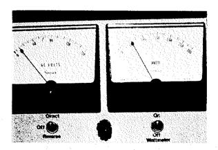
We've established the unit is drawing too much current. The power output transistors are the first components to check, since they are the most vulnerable to current overload. Checking transistors properly requires sophisticated test equipment. However, here is a practical transistor field test which only requires a VTVM set for reading resistance.
