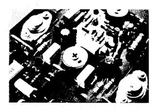
In the Model 250, the bias circuit consists of a diode, which is thermally coupled to the predriver to compensate for increases in temperature ...
