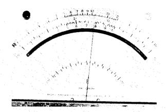
when the positive test lead is at the emitter or collector and the negative test lead is attached to the base. Reverse the test leads and resistance should increase to several megohms. This is because reverse polarity voltage is being applied.
