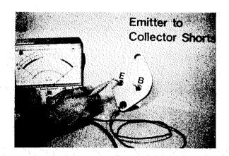
Resistance should be in the megohms when test voltage is applied in either direction.
