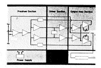
In most Marantz and Superscope power amplifiers, the bias voltage at the driver transistors is controlled by an adjustable bias control, which we'll check and adjust shortly. In most units a heat-sensitive bias protection circuit is incorporated with the bias control. It equalizes bias voltage on both driver transistors over the normal thermal operating range of the power amplifier.
