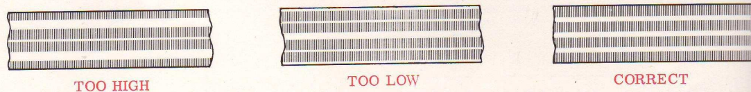
Fig. 3.7 Track measurement, 4-track record head.
