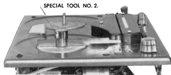
Fig. 19. Control of the horizontal position of the turntables with tool No. 2.
