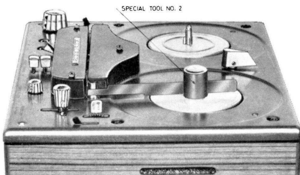
Fig. 19. Control of the horizontal position of the turntables with tool No. 2.
