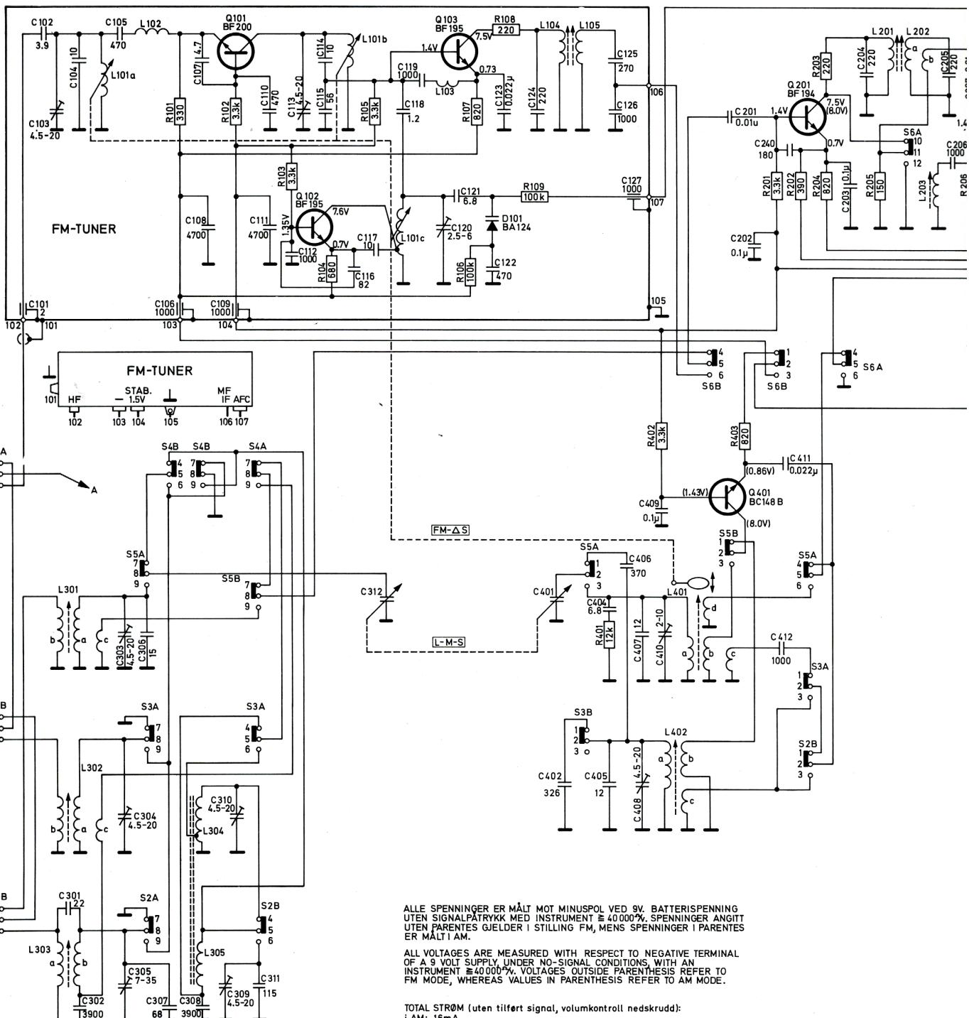
ALLE SPENNINGER ER MÅLT MOT MINUSPOL VED 9V. BATTERISPENNING UTEN SIGNALPÅTRYKK MED INSTRUMENT  $\geq 40\,000\%$ . SPENNINGER ANGITT UTEN PARENTES GJELDER I STILLING FM, MENS SPENNINGER I PARENTES ER MÅLT I AM.
