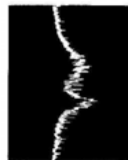
Fig. 14. 455 kHz felle (trap). Signal: U_{in} = 200 mV via wobbler/S.K.A. (fig. 15/16) tilført (applied) M14. Oscilloscope: Vert.: 50mV/div. Hor.: 2 kHz/div.
