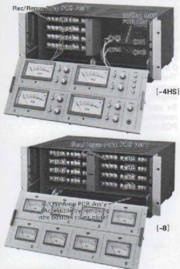
Fig. 9-5-8. Opening the Amplifier Module Front Panel
