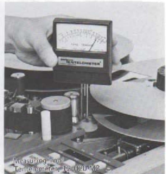
Fig. 9-4-7. Tape Tension Measurement and Adjustment Points
