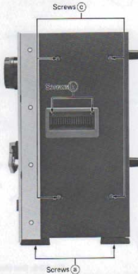
Fig. 9-3-3. Screw Locations for Side Panel Removal
